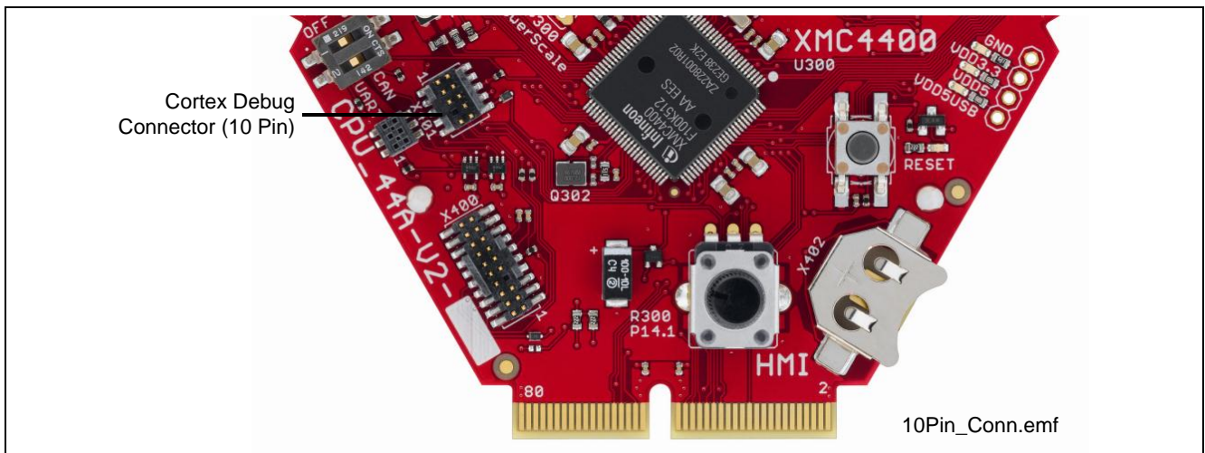
Figure 12 Cortex Debug Connector (10-pin) Layout
