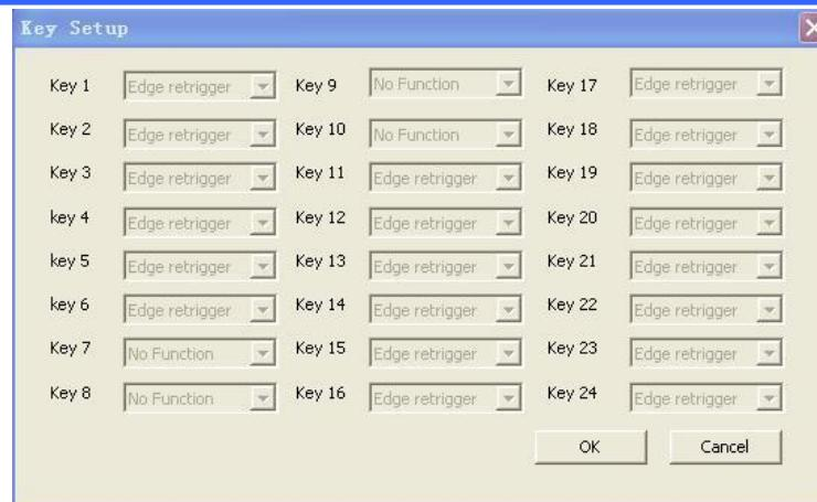
Open "Operation" "Equation", Key 1 to key 6 addresses were locked up. Others invalid.
