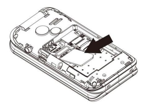
4. Install the battery as the following diagram show. Ensure the side with contactors faces down.
