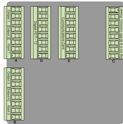
Back View Slot Orientation 1/4 DIN Horizontal PM4
