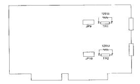
**CAN termination resistor installation**
