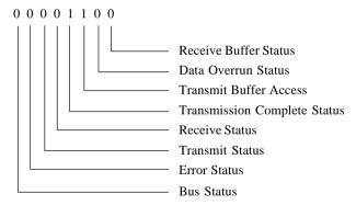
The registers can only be read if the CAN controller is in Normal mode. If the CAN controller operates correctly and the transmission has been completed successfully, the status register will show as the normal value: 00001100. If the Error Status and/or the Bus Status is 1, you have selected the wrong baud rate or the CAN cable is damaged. Also check the correct bus terminator.
