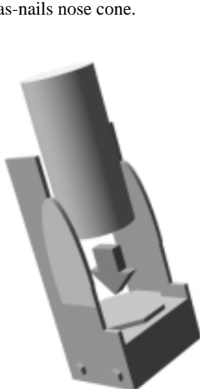
Mount the plug of foam to the rotating base plate with double-sided tape.
