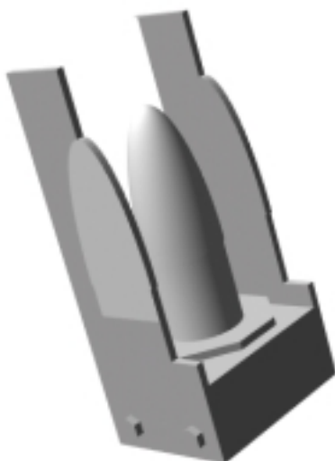
With enough passes of the wire, the nose cone will come out nearly perfect and is ready for finishing.
