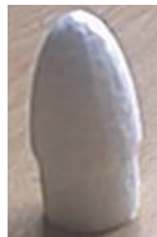
Fire up your hot wire foam cutter, and use the side templates to guide the wire as you cut through the foam. Rotate the nose slightly, and repeat this cutting procedure. Make sure to keep the wire moving, or you could melt a divot into the side of your nose cone.
