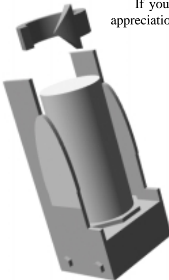
Make sure the foam can rotate freely between the side plates
