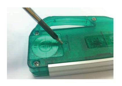
Remove Screw to remove battery from the compartment
