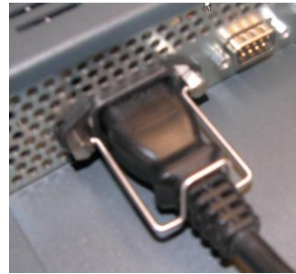
Power Cable Retention Clip Installed
