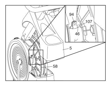
Locate the Reed Switch (46). Turn the Pulley (58) until a Magnet (107) is aligned with the Reed Switch. Next, loosen, but do not remove, the indicated M4 x 13mm Flange Screw (94). Slide the Reed Switch slightly closer to or away from the Magnet, and then retighten the Screw. Turn the Pulley for a moment.
