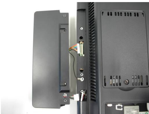
b. Connect the MSR cable and slide the MSR into position
