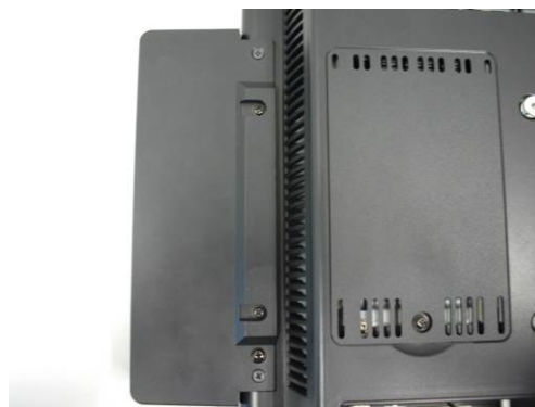
c. Connect the MSR module to the system and tighten the screws (3)
