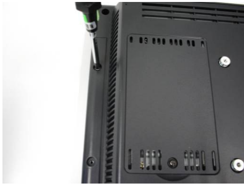
a. Loosen the screws (2) on the MSR dummy cover
