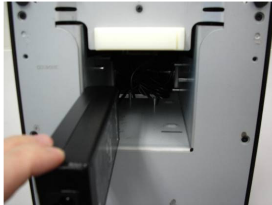
d. Remove the adaptor from the stand
