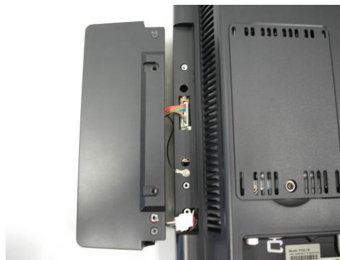
b. Connect the MSR cable and slide the MSR into position
