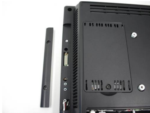
a. Loosen the screws (2) on the MSR dummy cover
