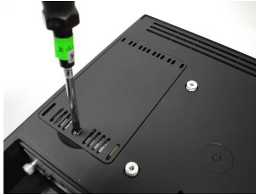
a. Loosen the screw * 1
