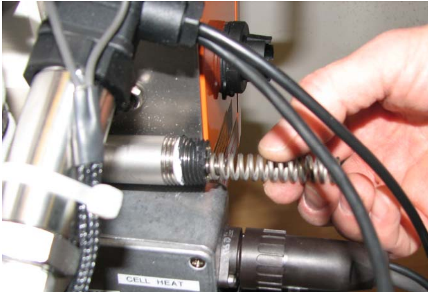
Figure 21 – Removing the Spring from Course Filter Tube
