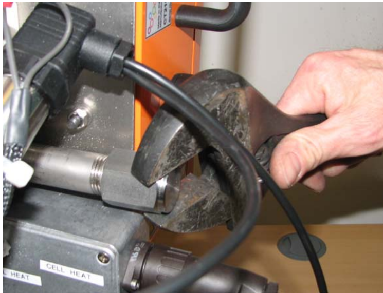
Figure 20 – Removing the End Cap from Course Filter Tube
