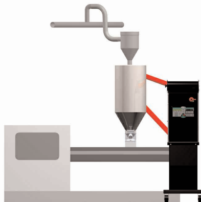
Dryer on a floor stand; hopper on the throat.
