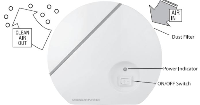
To use the Ionising Air Purifier, plug it into any standard electrical outlet and switch the unit on. The power indicator light will show if there is a power supply.
