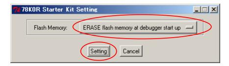
③Now, start the debugger. As you erased the flash memory with above processes, you need to enter "FFFFFFFFFFFFFFFFFF" (F x 20) in ID code on the configuration window of the debugger.
