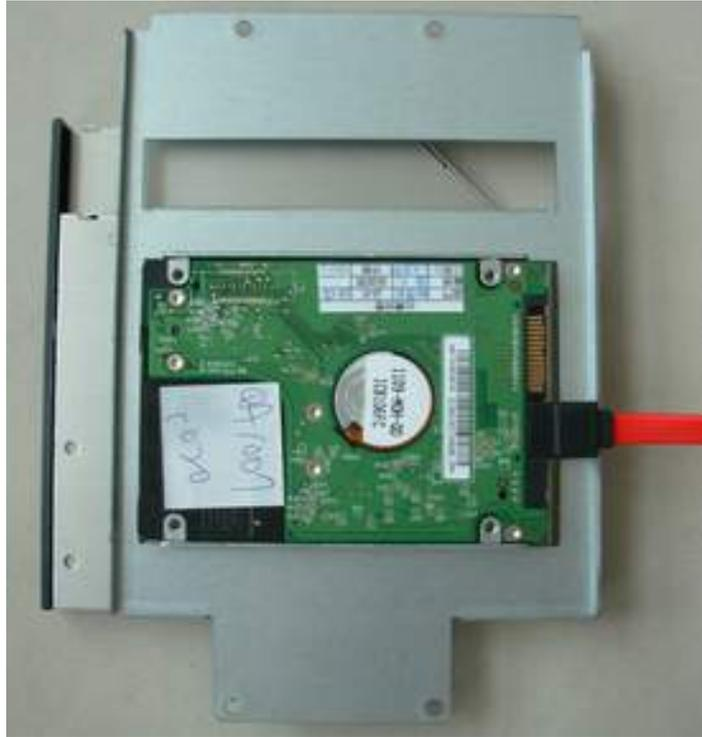
17. Turn the CD-ROM driver screws and SATA cable connects well and turn the screws..
