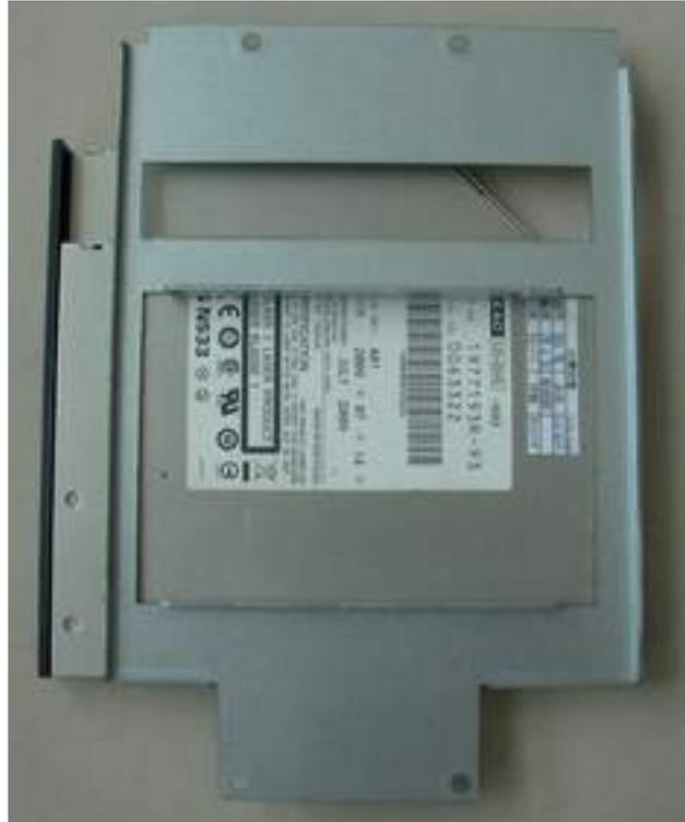
Put on HD driver into HD holder then turn the HD drive screws to tighten. Refer picture A , B and C.
