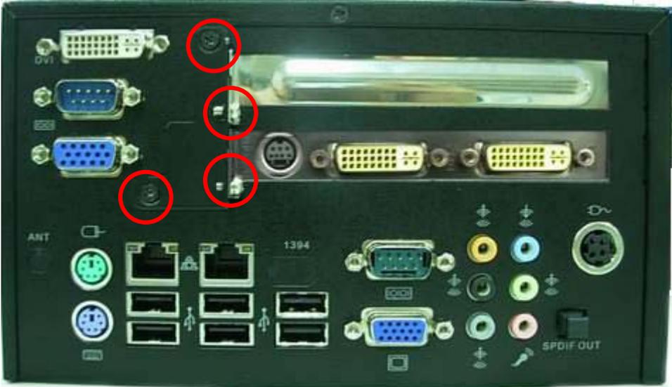
10. After install HD driver, Turn the CD-ROM holder and front panel screw well refer picture.
