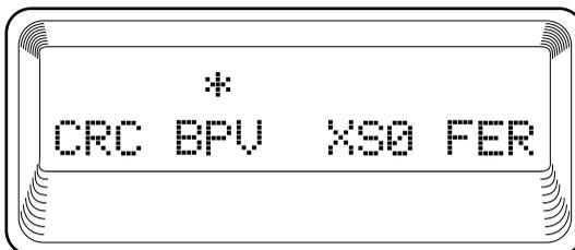
**Figure 3-4. D & I Errors Display**
