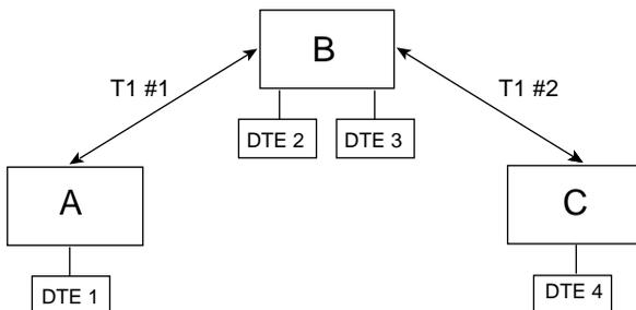
**Figure 1-1. D & I Used With Two Separate T1s**
