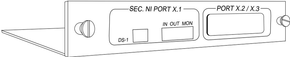
**Figure 1-2. Full Drop and Insert Option Module**
