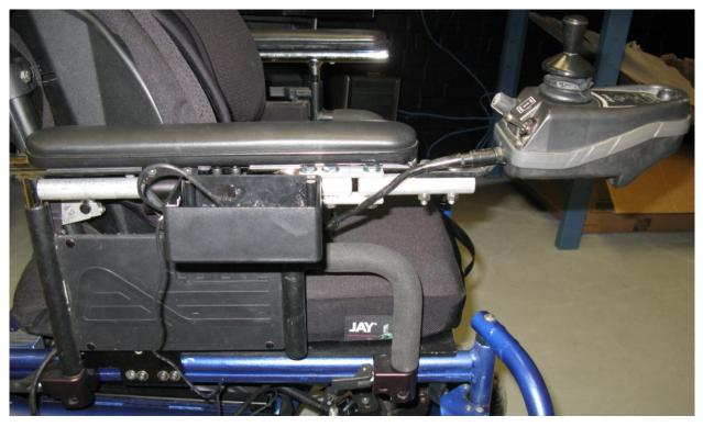
To the right armrest, there is a bar attached, and the actuation control box is screwed to this bar. The end of this bar is then connected to a shorter bar to which the joystick is held. These two bars are held together by a piece of aluminum above and below the bar that is screwed in. The bars are far enough apart to allow 90° rotation of the front bar, thereby forming a hinge.
