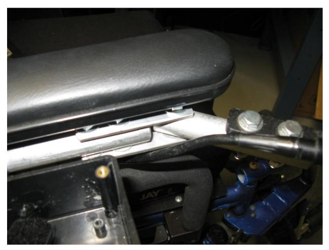
The seat base plate also sits on the side rails and is secured by six screws. On top of the seat base plate is Velcro to which the seat cushion is attached.
