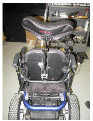
The headrest attachment is connected to the aluminum seat case via four long, threaded screws that prevent excess torque on one screw and hold it in place securely.
