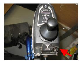
• Activate the tilt sensor by toggling the switch labeled tilt sensor to the right.
