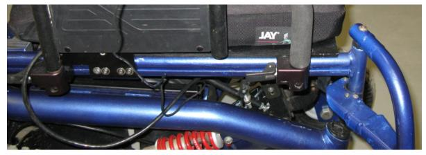
The back mount cross bar is connected to the side rails via screws that go through the two holes on either side of the cross bar and into dove tails in the side rails. The harness and seat belt are also attached to the side rails in this manner.
