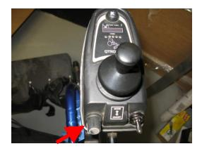
• Push the joystick forward to move the chair forward. These controls work for side to side and reverse as well.
