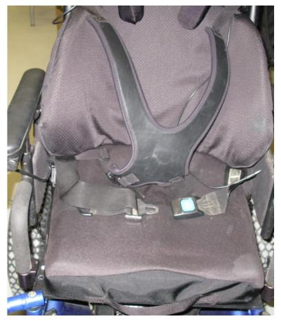
The back cushion is attached to the plastic seat case by velcro that lines a large area of both pieces.
