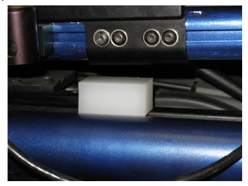
The motor mounts are attached by large bolts into the tube at the bottom of the chassis, and are also secured on by the shocks which attach to the top of the motor mount and connect to the underside of the upper chassis by a bolt. The motors are attached to the motor mounts by four bolts on the bottom of the mount cage.
