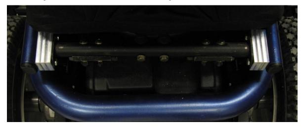
The front cross bar resides between the front two spacers and the rear cross bar resides between the back two spacers. They are held in place by the same screws that hold the spacers tightly. The cross bar connector is screwed into two holes in each cross bar and gives the overall seat mount assembly stability.
