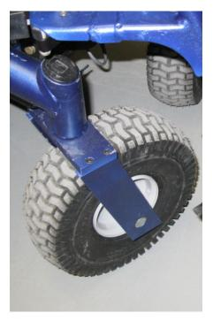
There is also a hole at the bottom of each angular piece, one of which is threaded, to allow a bolt to pass through one side, go through the front wheel, and screw into the other side. This attaches the tire to the caster. Between the inside face of the caster and the tire there is also a caster spacer that helps prevent the tire from sliding along the bolt.
