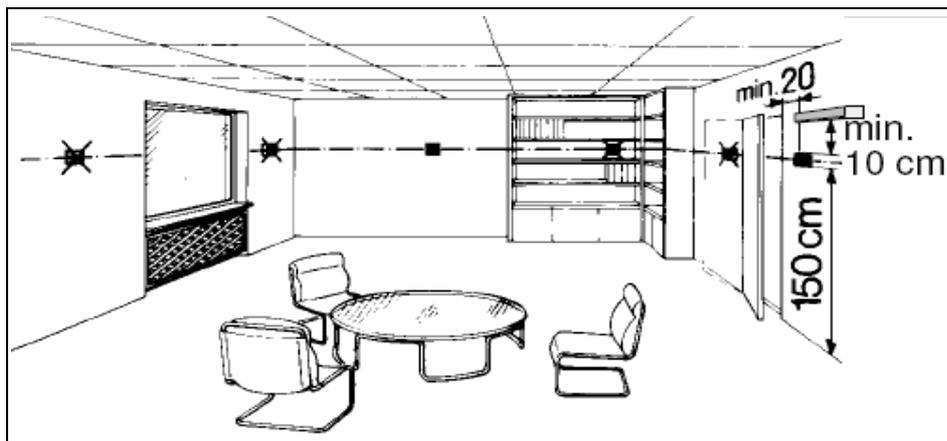
Figure 16 Installation position of the QAA78 room unit.
