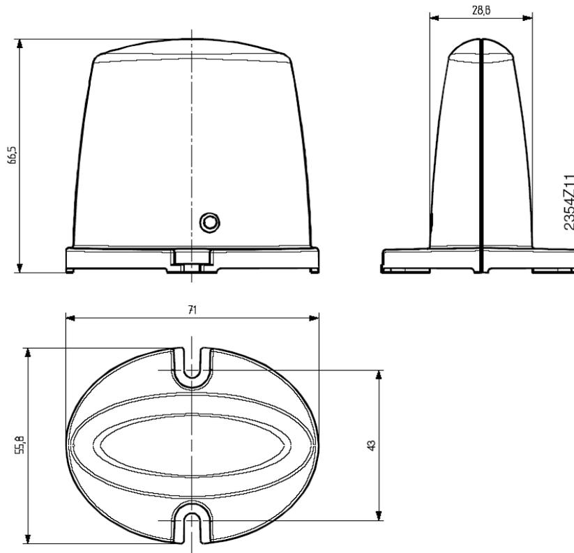
Figure 15 AVS71 radio module drilling holes.
