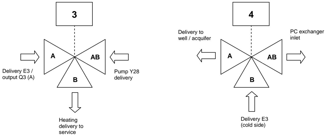
**Figure 38** Description of direction of flow of valves n.3 and 4 shown in Figure 35.
