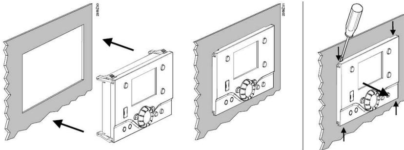
**Figure 4** Installation method
