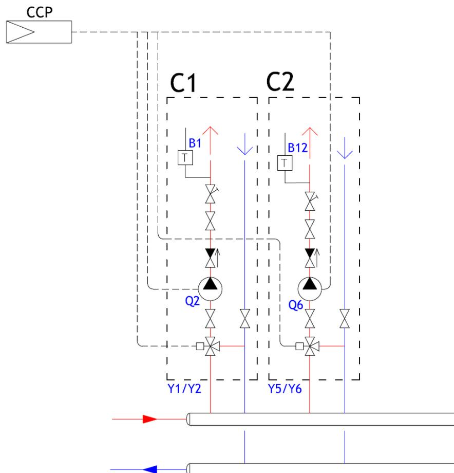
**Figure 53** Mix 1 and 2 circuit components
