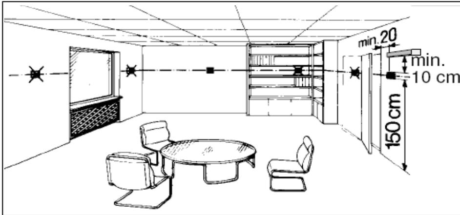
**Figure 11** Installation position of the QAA75 room unit.
