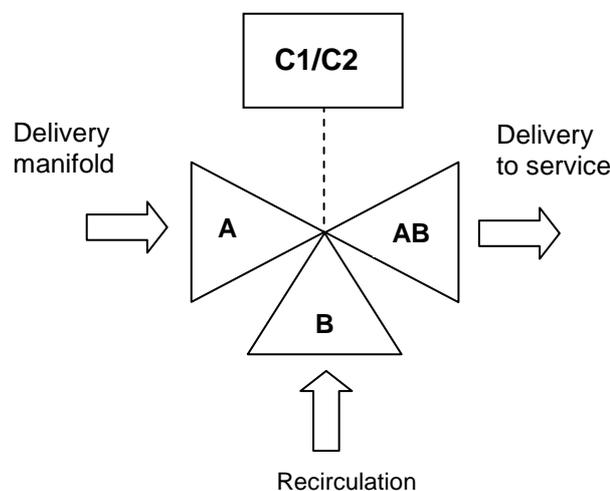
**Figure 42** Description of direction of flow of mixer valves
