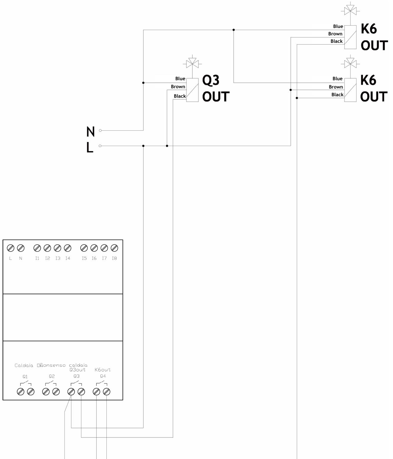
**Figure 32** Diverter valves Q3 connection<sub>OUT</sub> and K6<sub>OUT</sub> directly from PLC
