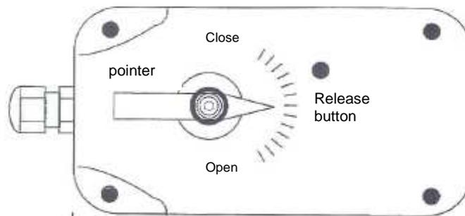
**Figure 40** Description of actuator: The “pointer” indicates and controls the position of the actuator in Figure 39, the “release button” is used for moving the “pointer” by hand.
