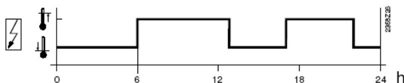
**Figure 60** Time program 4/DHW. The symbol
