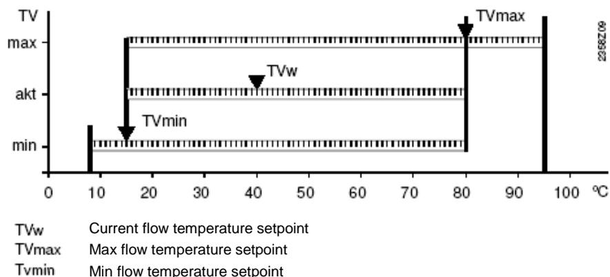
**Figure 63** Description of delivery water temperature limits
