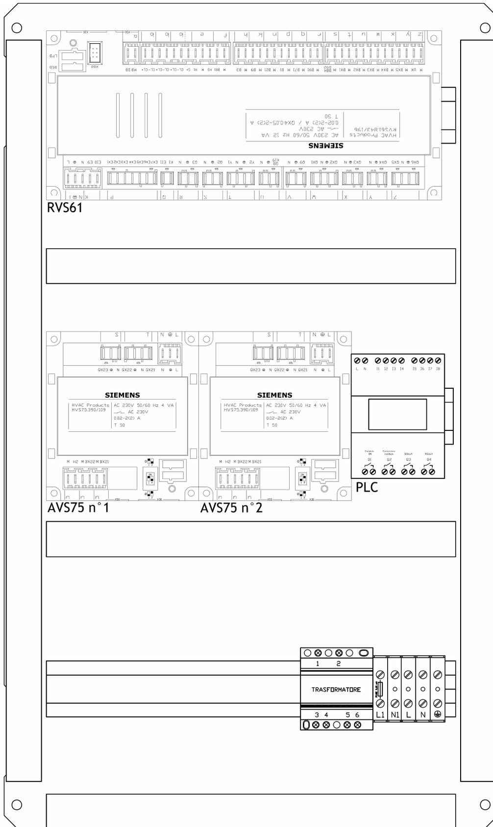
Figure 2 Comfort Control Panel (CCP) layout
