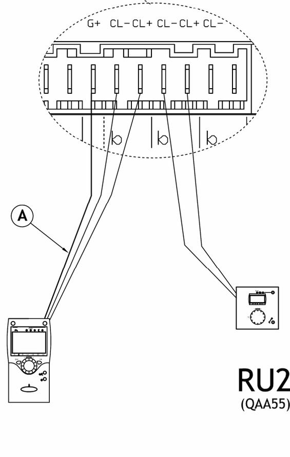
**Figure 26** Example of backlighting connection on room unit (QAA75.. with backlighting)
