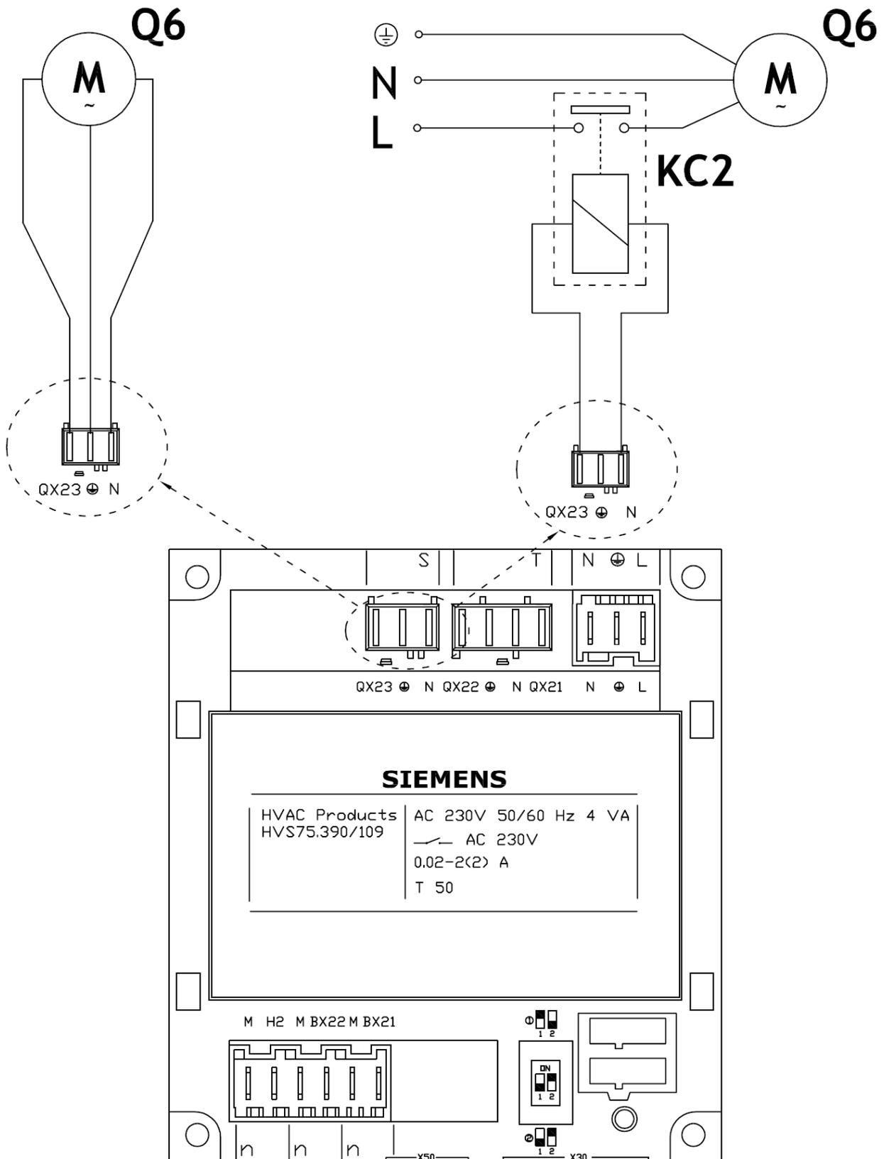
**Figure 29** Direct or externally relayed connection to heating circuit 2 pump on expansion module n.2.
