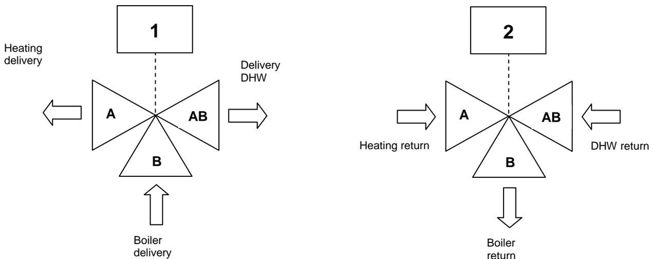
**Figure 37** Description of direction of flow of valves n.1 and 2 shown in Figure 35.
