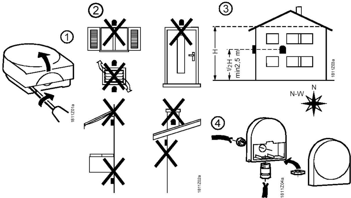
Figure 5 Installing the QAC.34 external sensor
