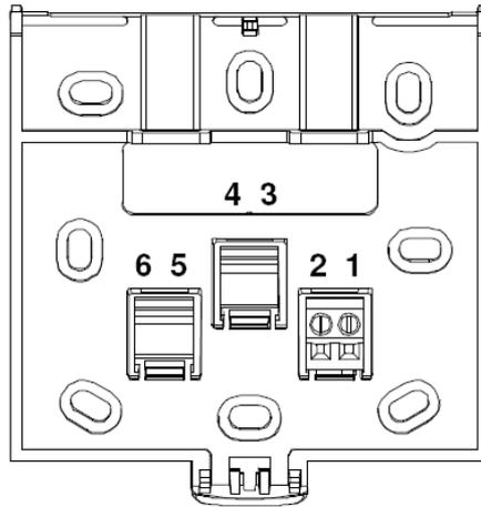
**Figure 9** Connection of the QAA55 room unit.
