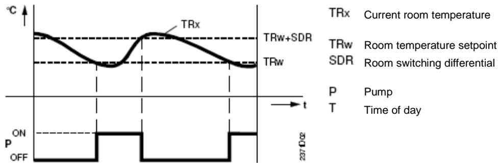
**Figure 65** Example of pump operation depending on the internal room temperature setting
