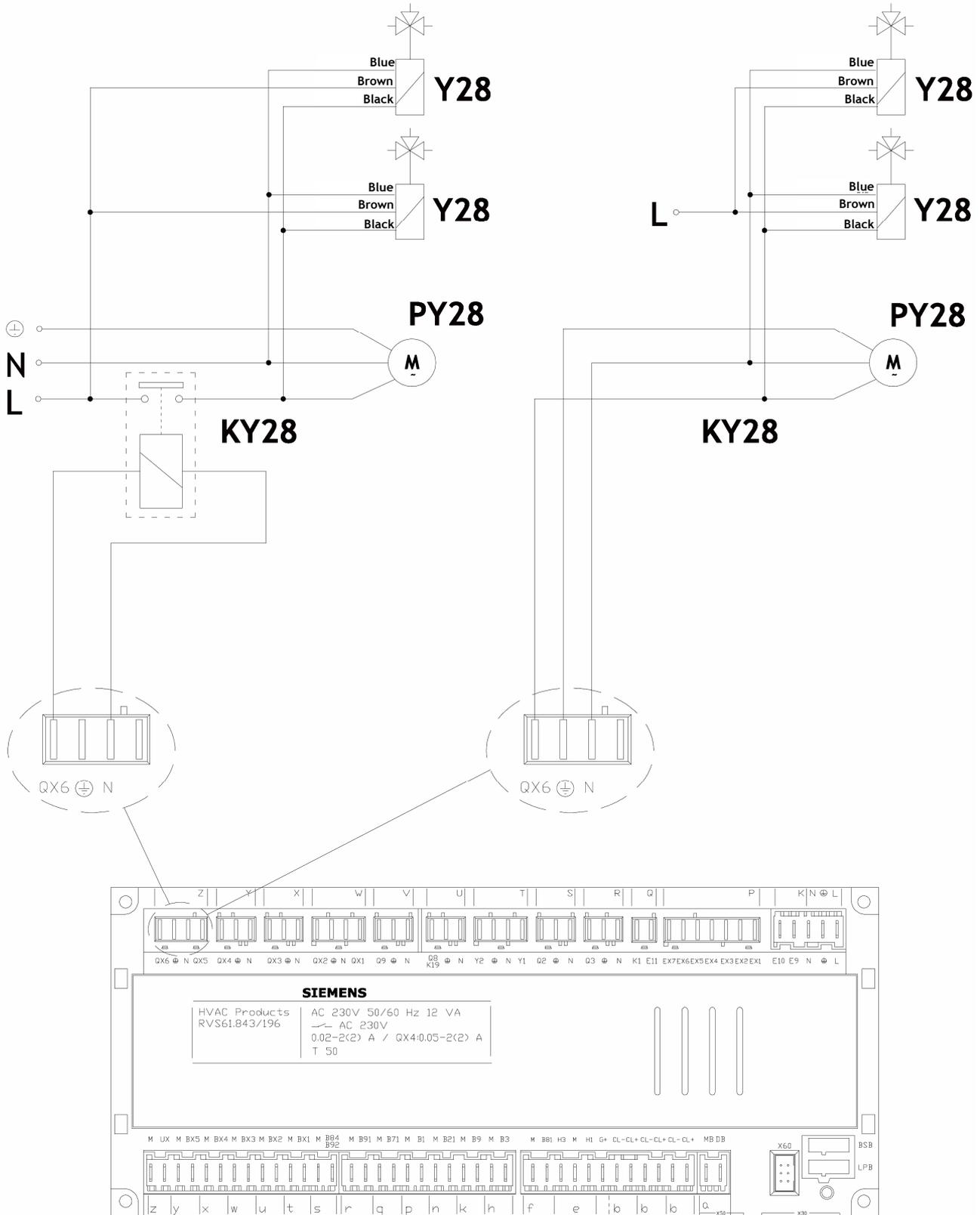
Figure 31 Direct and relayed connection of diverter valves Y28 and pump PY28
