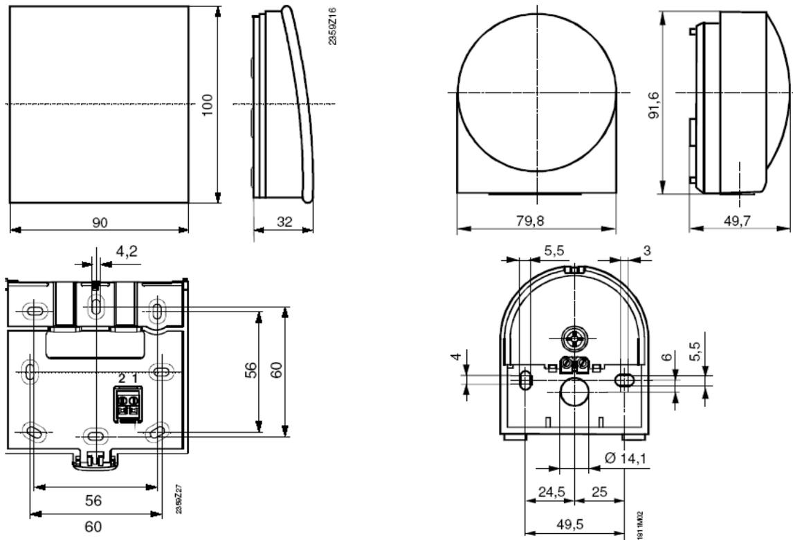
Figure 22 External radio sensor drilling holes.
