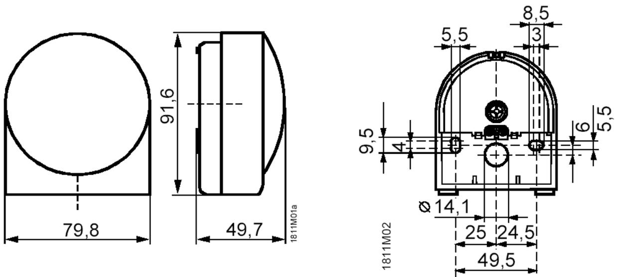
Figure 6 Dimensions of the QAC.34 external sensor
