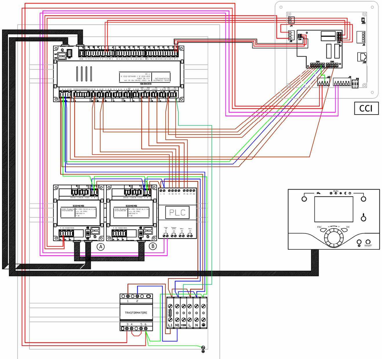
Figure 3 Comfort Control Panel (CCP) wiring diagram
