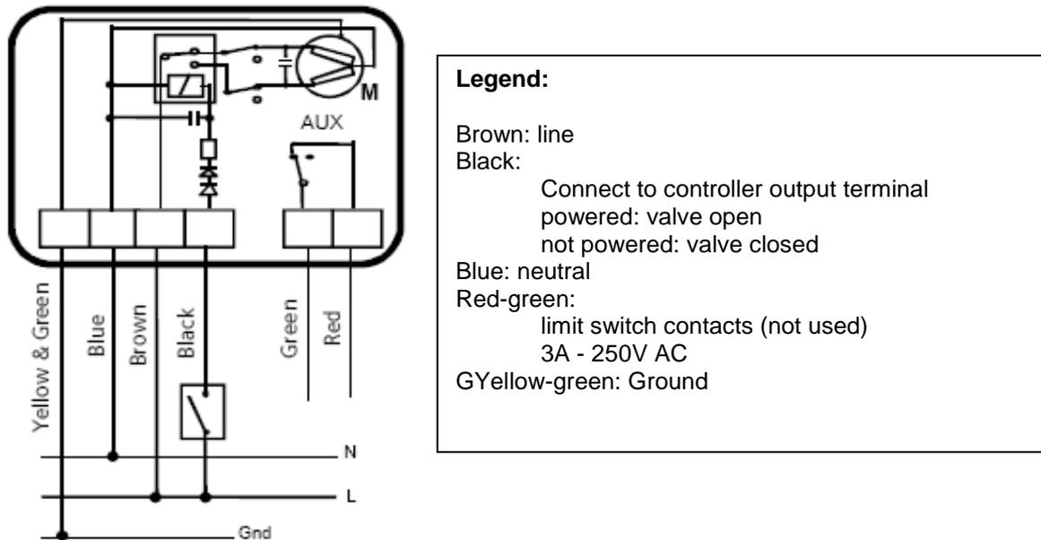
**Figure 41** Description of diverter valves actuator connections
