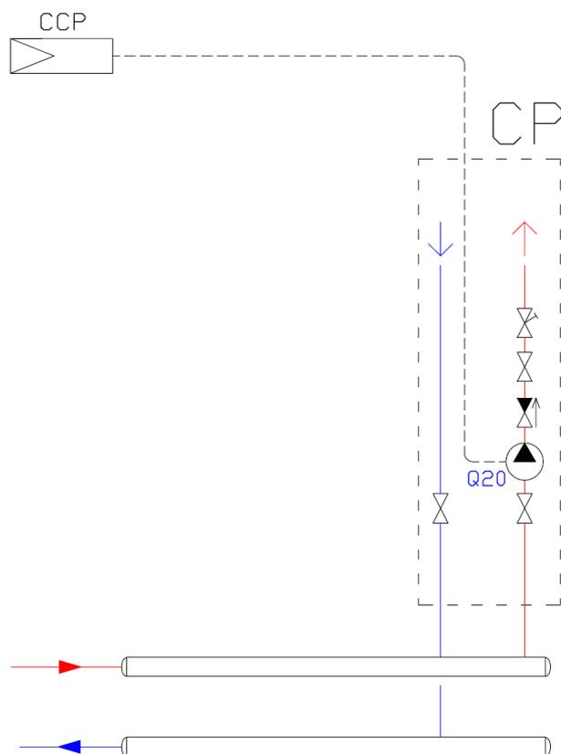
**Figure 54** Pump circuit components
