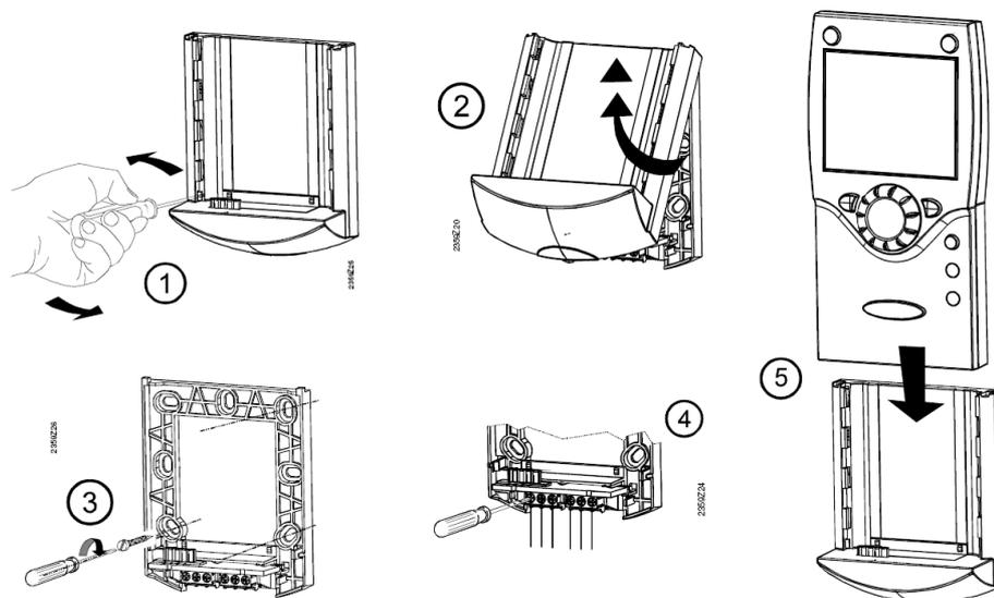
**Figure 12** Installation of the QAA75 room unit.
