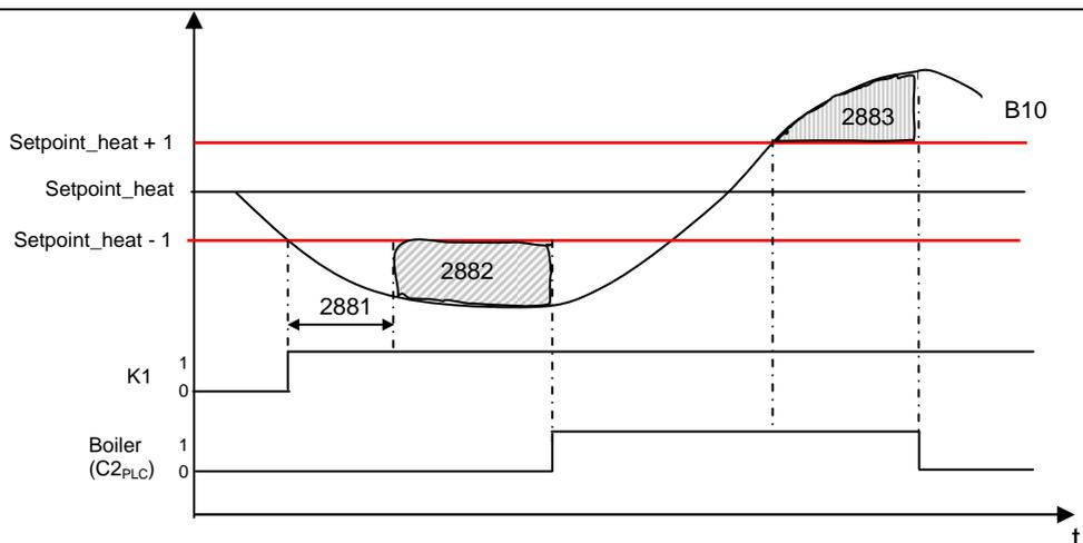
**Figure 61** Supplementary heating boiler activation graph.
