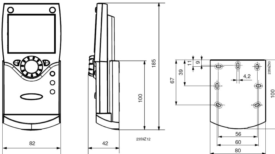
**Figure 13** QAA75 room unit drilling holes.
