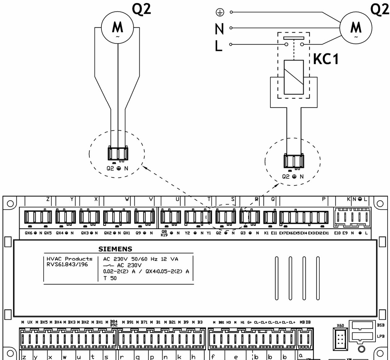
Figure 28 Direct or externally relayed connection to heating/conditioning circuit pump on RVS61.
