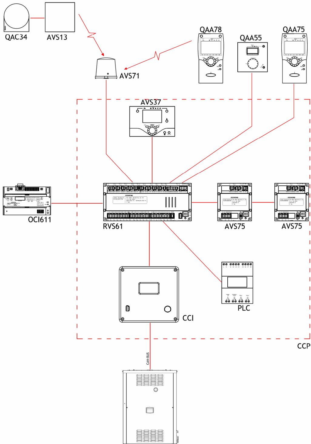
**Figure 1** Comfort Control system components
