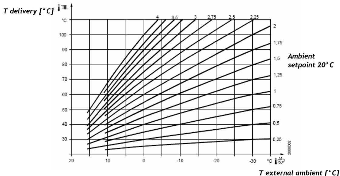
**Figure 62** Heating curve graph. The figure shows a family of heating curves with various slopes (0.25 to 4). Each curve characterised by its slope, represents the delivery v. the external ambient temperature, when the required setpoint is 20°C.
