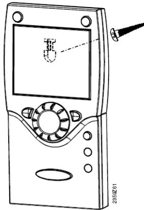
**Figure 18** Installation of the QAA78 room unit.
