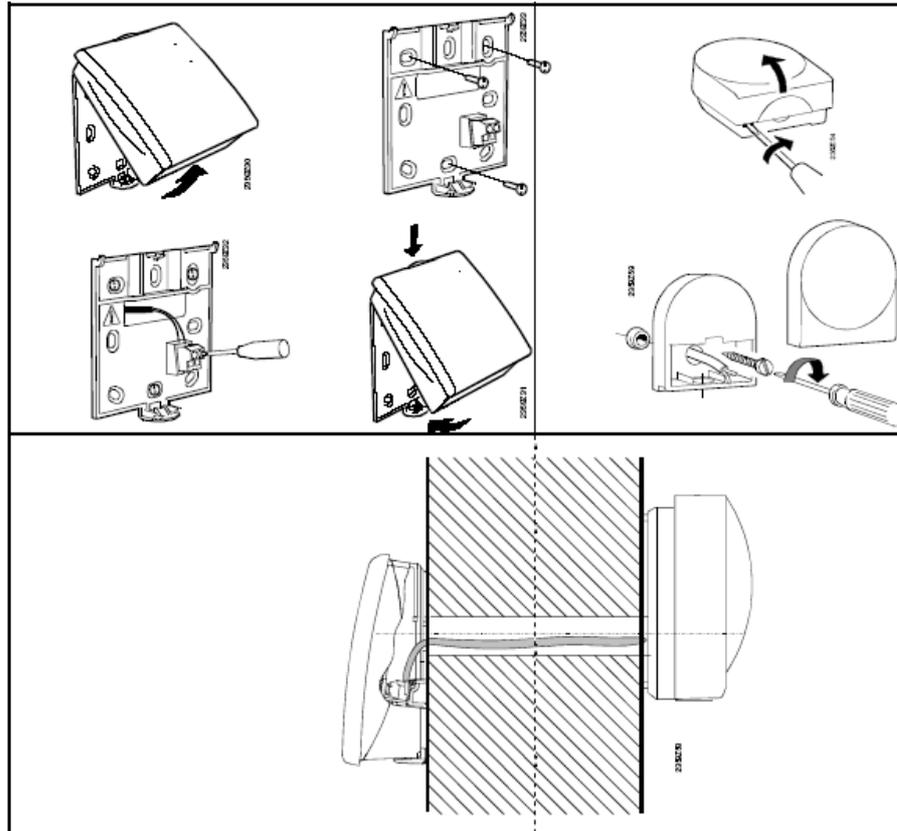
Figure 20 Installing the external radio sensor.
