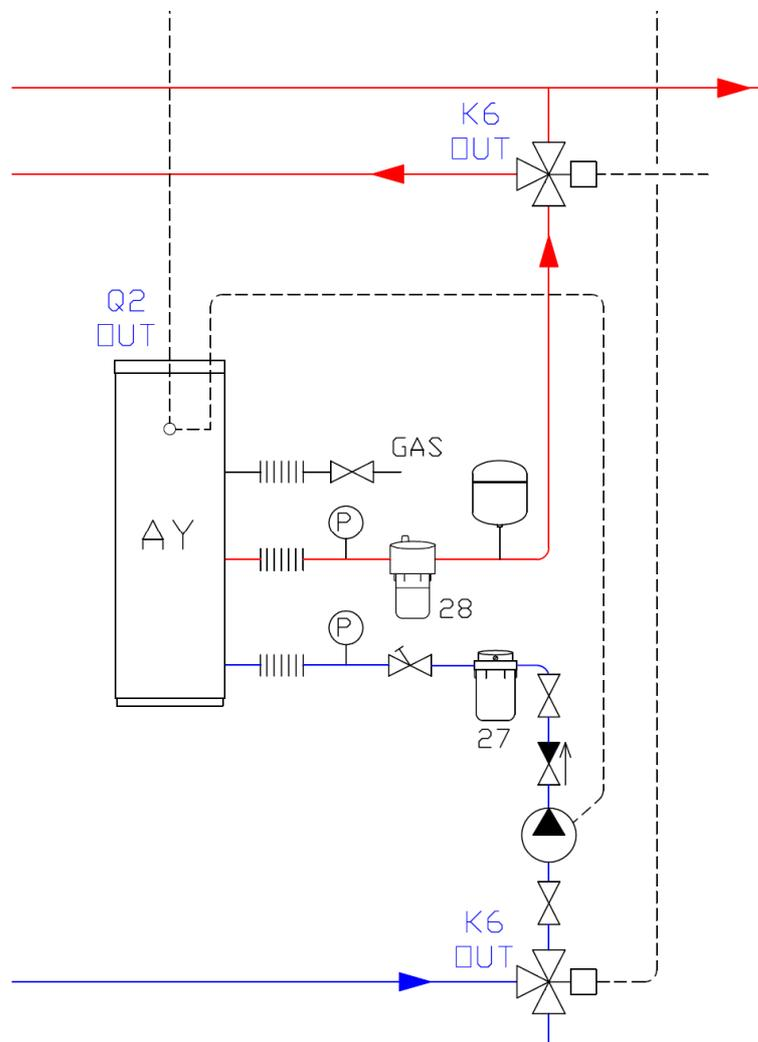
**Figure 52** Heating/DHW supplementary boiler components.
