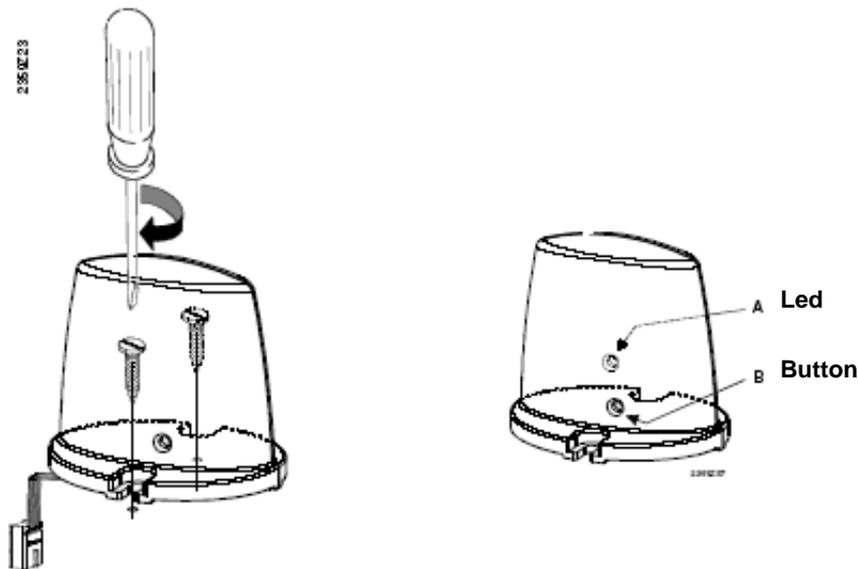
**Figure 14** Installation of the AVS71 radio module.
