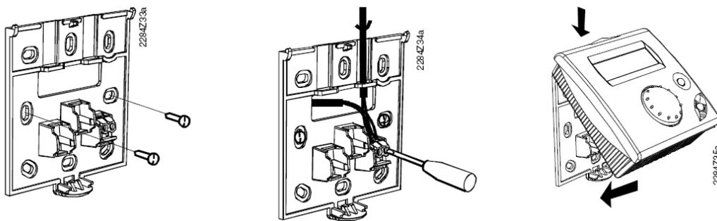
**Figure 8** Installation of the QAA55 room unit.
