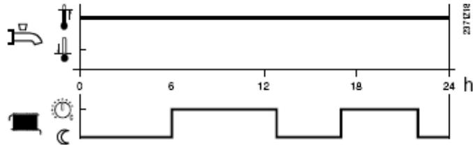
Set “1620: Release” to “24h/day” to ensure that the heat source can always be used for DHW at the “Nominal setpoint” (if requested by the service), but heating service may be compromised. To “balance” the use of the heat source for heating and DHW, use parameter “5030: Charging time limitation”.
