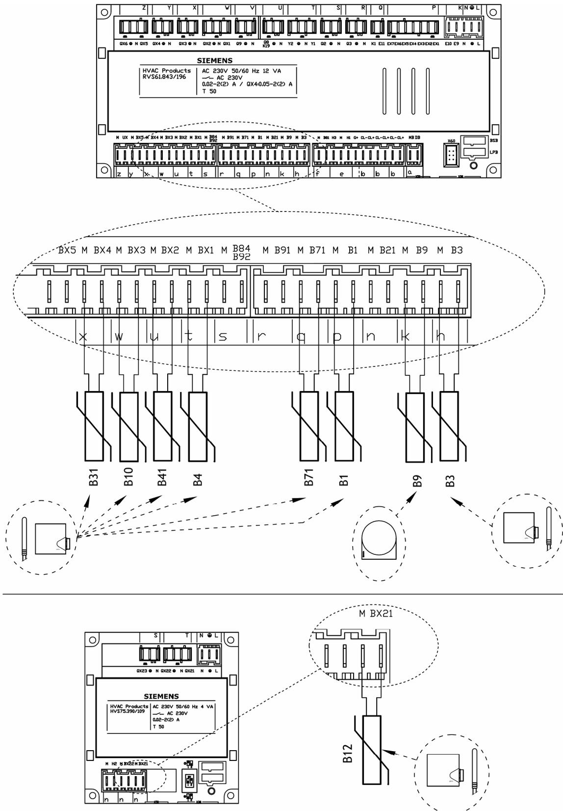
**Figure 27** Example connection of temperature sensor connection to RVS 61 and expansion module AVS75.
