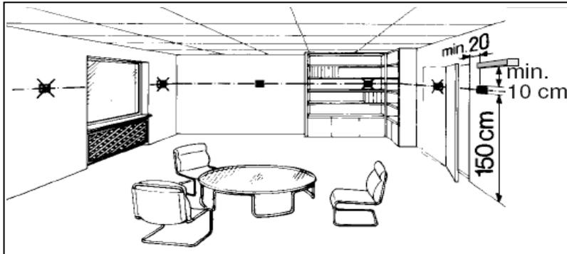
**Figure 7** Installation position of the QAA55 room unit.
