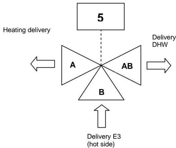
**Figure 36** Description of direction of flow of valve n. 5 shown in Figure 35.
