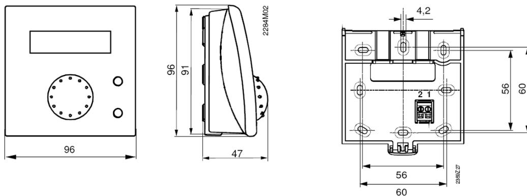
**Figure 10** QAA55 room unit drilling holes.
