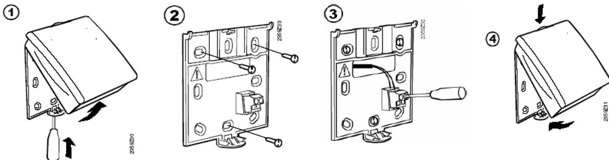
Figure 23 Installing the radio relay.
