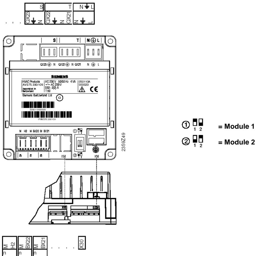
Figure 25 Identification of modules 1 and 2
