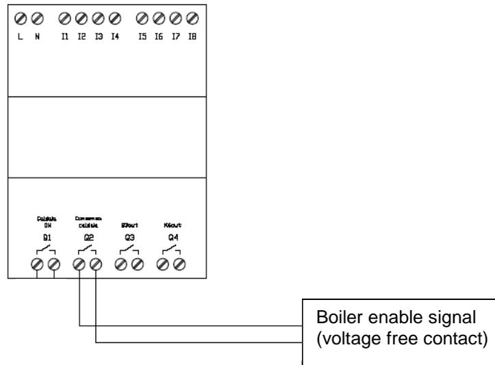
**Figure 34** Heating/DHW supplementary boiler On/Off signal connection.
