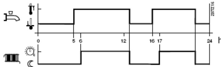
Set “1620: Release” to “Time programs HCs” to ensure that, when operating with Comfort heating mode, the heat source can always be used for DHW at the “Nominal setpoint” (if requested by the service), but heating service may be compromised. To “balance” the use of the heat source for heating and DHW, use parameter “5030: Charging time limitation”.
