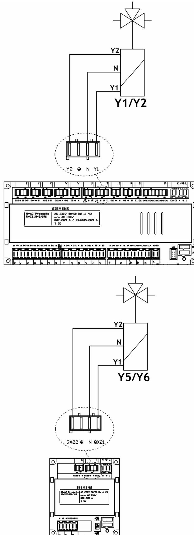
Figure 33 Mixer valves Y1/Y2 (circuit C1) and Y5/Y6 (circuit C2) connection
