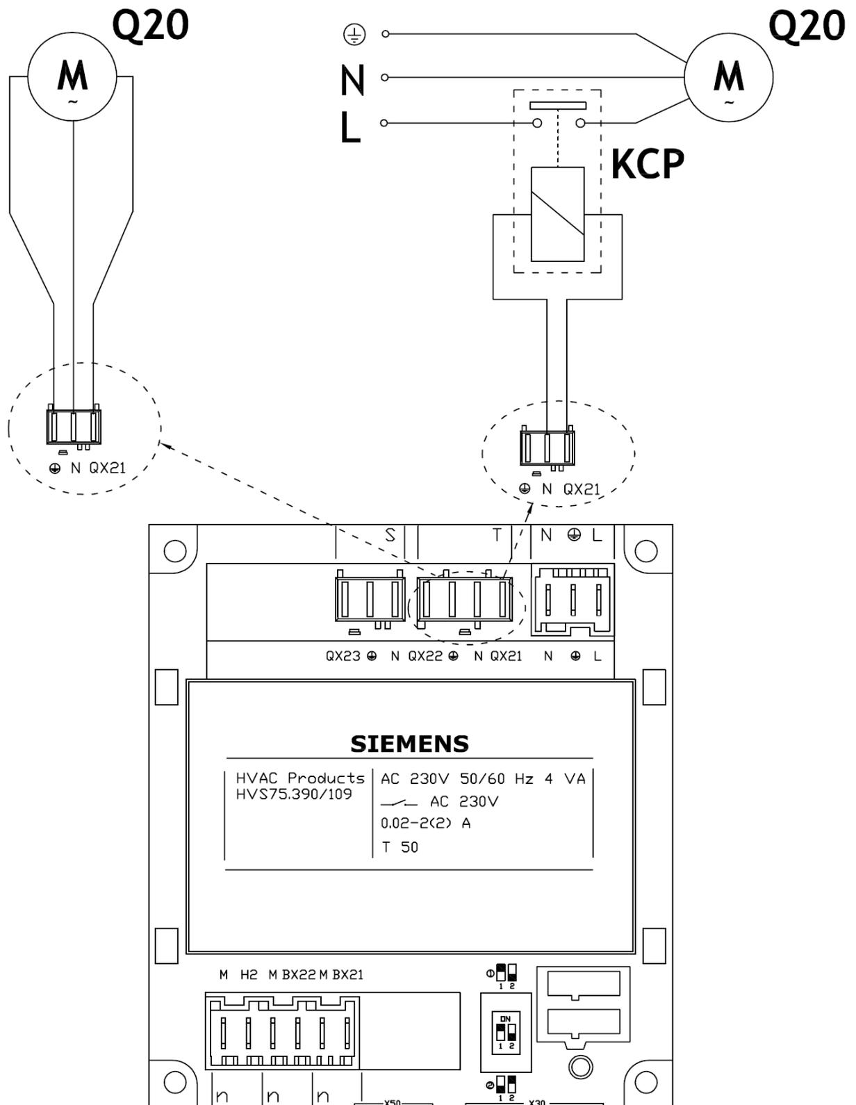
**Figure 30** Direct or externally relayed connection to heating circuit P pump on expansion module n.1.
