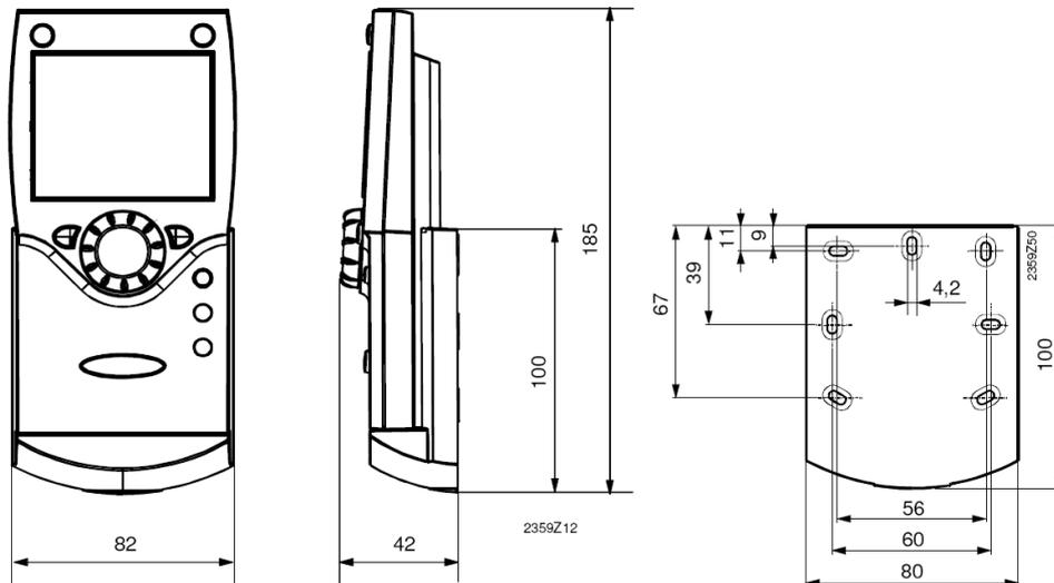
**Figure 19** QAA78 room unit drilling holes.
