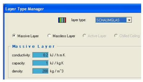
Figure 6.6 Input parameters in TRNBuild for the thermal characteristics of the various material layers
