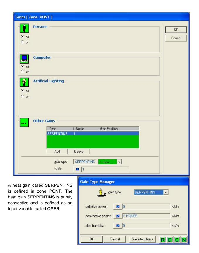
Figure 6.7 Input parameters in TRNBuild for the definition of the input convective heat gain in the zone PONT
