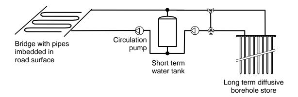
Figure 5.2 Simplified system layout of the Serso plant, equivalent to the one simulated by the BRIDGESIM tool.
