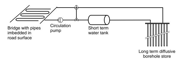
Figure 5.1 System layout simulated by the BRIDGESIM tool.
