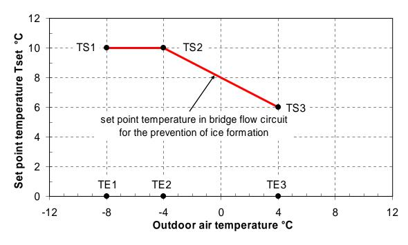
Figure 5.3 Control of the forward fluid temperature in the bridge in function of the outdoor air temperature when the system operates in the ice prevention mode (bridge heating).
