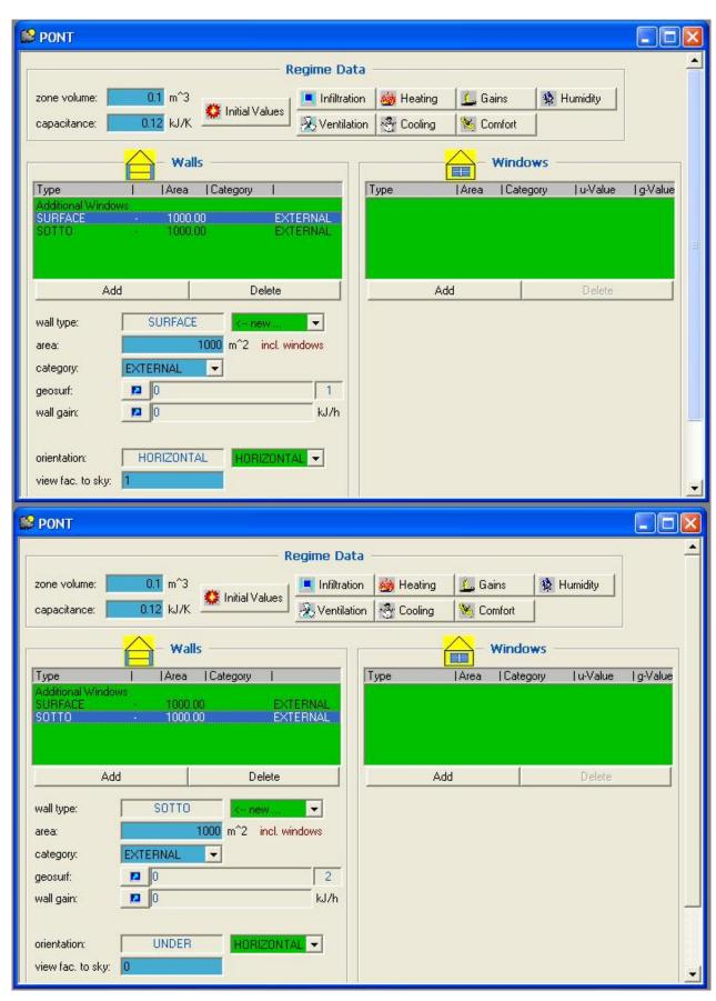
Figure 6.3 Input parameters in TRNBuild for the two walls SURFACE and SOTTO of the thermal zone PONT. They have to be defined in this order so that wall 1 is wall SURFACE and wall 2 is wall SOTTO.
