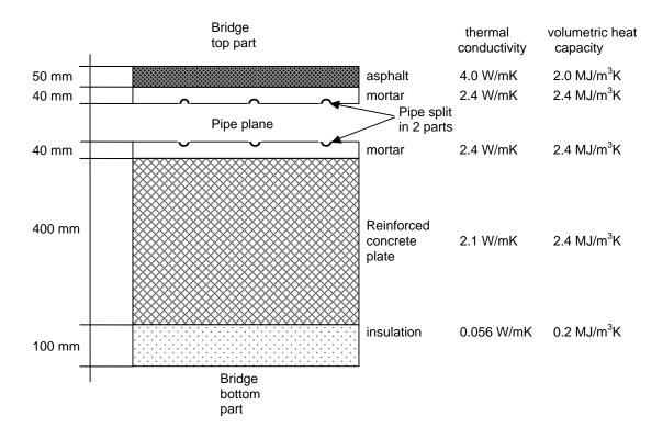
Figure 6.1 Section of the bridge in Serso subdivided into two parts: above and below the pipe plane
