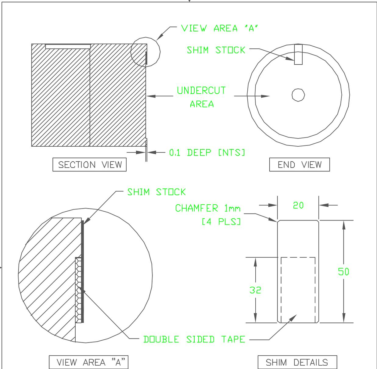
1. THOROUGHLY CLEAN AND DEGREASE AREA WHERE SHIM IS TO BE FITTED.
