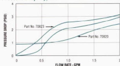
Tests conducted with units in a vertical position (lead wires up), with water at +70°F
