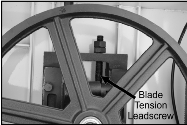
Figure-36 Lubricating the blade tension lead screw
