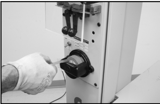
Figure-23 Grinding the blade ends
