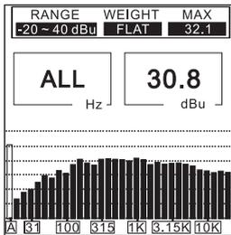
Measure the line voltage level in units of dBu, dBV, and voltage, using standard response time, and standard A, C, and flat weighting network (Under normal condition, please set it at Flat). MPAA1 can only measure AC voltage; if user measure DC voltage with MPAA1, it may damage MPAA1 and hence void the warranty.
