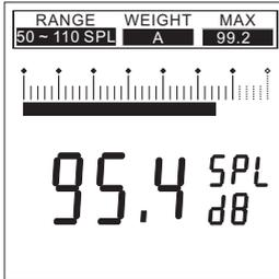
Measure the loudness of the ambient sound level in units of dB SPL. This is a true RMS-measurement, using standard display time average, and standard A, C, and Flat weighting network.
