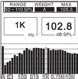
Analyze the audio received through the built-in omnidirectional mic by dividing the audio spectrum into 31-band, 1/3 octaves, and displaying a bar graph that shows the dB level of each band of sound from 20Hz to 20KHz in four different response time (35ms, 125ms, 250ms, and 1sec) and in three weighting types (A weighting, C weighting and Flat).
