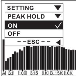
Peak hold of the selected unit being measured could also be shown constantly on the LCD screen. It tells you the peak value of each frequency and all frequency in RTA mode.
