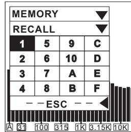
User can recall all the data saved in the memory of MPAA1, to make comparison or and see the difference between (among) the measurement.
