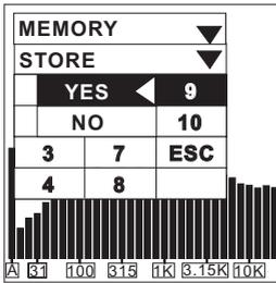
User can save up to 10 set of measured data, as well as 6 other averaged one, into the memory of MPAA1 for further analysis or uploading.
