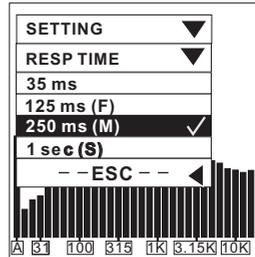
For different kinds of measuring purpose, different setting of response time is needed for the measurement.
