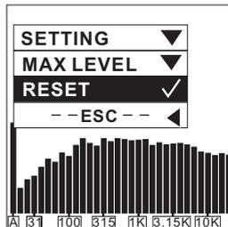
Maximum level will always be measured and shown constantly on the LCD screen. It is recommended to reset the max level before each new measurement.
