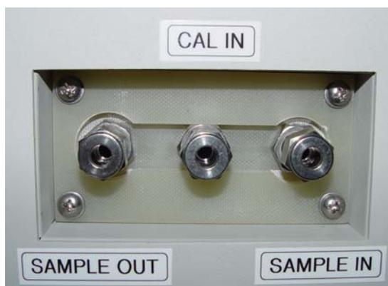
Figure 3 - Gas connections
