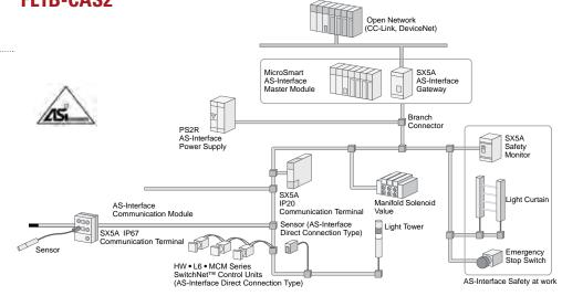
Primarily for control of sensors and actuators at distances of up to 100 meters, this interface utilizes the simplest and most-effective programmable control based industrial networking protocols, used in automation systems worldwide. Reducing the amount of engineering by employing simpler wiring, this module also enhances your operations by requiring little to no maintenance.
