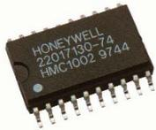
Honeywell's magnetoresistive sensors are able to sense Earth's magnetic field (~0.6 gauss) and provide the sensitivity for enhanced accuracy and performance. Honeywell offers 1-, 2- and 3- axis magnetic sensors for low field linear applications and small size.
