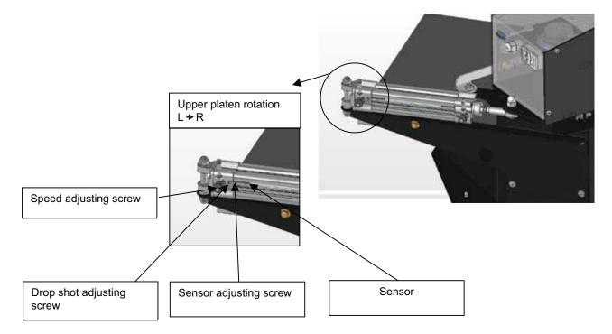
By means of a screwdriver, periodically adjust the swinging speed. It varies as a function of lubrication and wear of mechanical parts.
