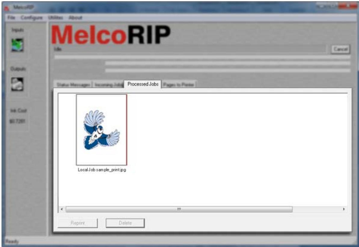
This view will allow the user to view and manipulate jobs which have been processed and have not yet expired (expiration time is set in the “Configure MelcoRIP” option under the “Configuration” menu item).
