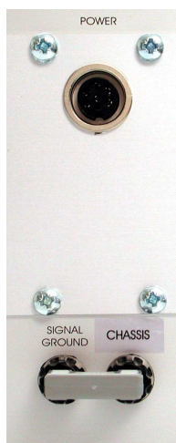
Figure 4: Rear panel connectors of the EPMS-E-07
