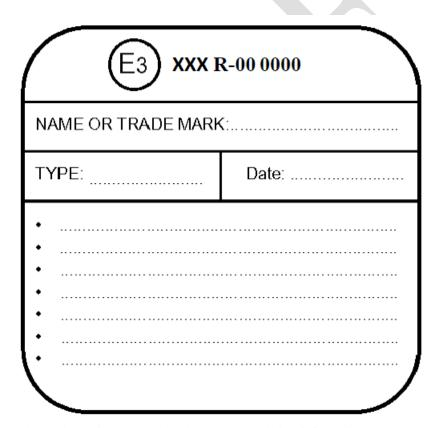
The above plate, with approval mark and some technical information on the HDDF retrofit system, has to be permanently fixed on the body of the vehicle.
