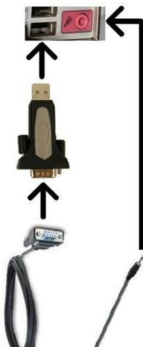
*This picture shows how to connect the “serial lead with audio jack (IV)” to the “USB to serial adaptor” (II) and then to your computer’s USB port and microphone socket.*
