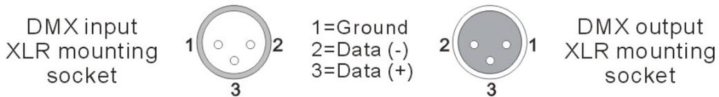
If you are using controllers with this occupation, you can connect the DMX-output of The controller directly with the DMX-input of the 1st device in the DMX-chain. If you wish to connect DMX-controllers with other XLR-outputs, you need to use adapter-cables.
