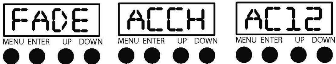
Press the Menu button. Press the Up or Down button until it shows one of the following:
