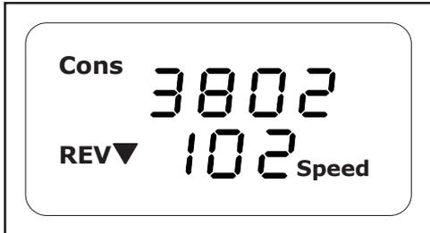
1. Press **CONSIST** then **LOCO**. Make sure "Cons" appears on the LCD display.
