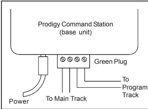
1. Using a small flat-bladed screwdriver, attach two wires (22 AWG or heavier) from the Main Track layout to the terminals marked Main Track and two wires from the Program Track to the terminals marked Program Track.
