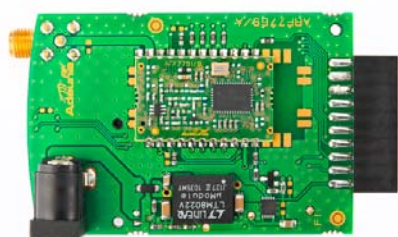
Adeunis RF Wireless M-Bus extension board
