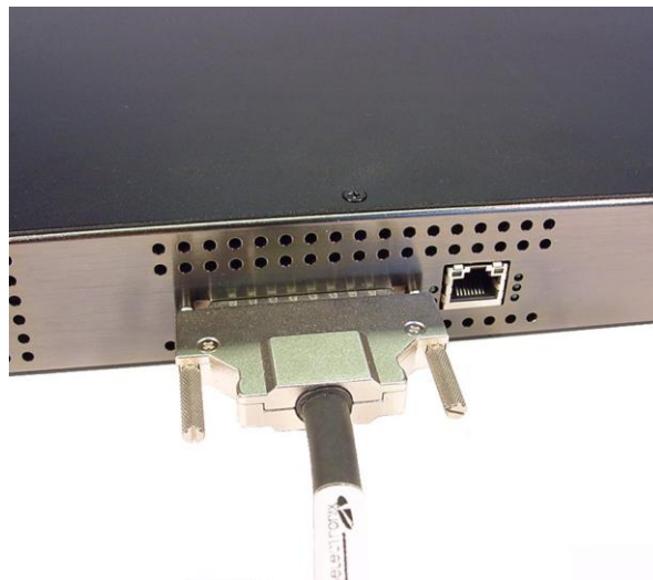
Connecting the SCSI Cable to the Bridge SCSI Port
