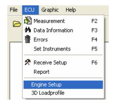
This window called by "ECU Mode", and allowed to set the ECU in "All speed governor- or Torque Mode" (=default). To change this Mode, the engine have to operate in ignition (no running engine), window confirm the changing mode. Engine Setup "Mode change" is only in MARINE version available.
