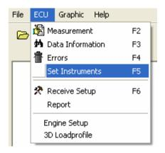
This window is called by "ECU -> Set Instruments" in the Menu or with hard key "F5". This function allows to calibrate the instruments and set the idle speed between 600rpm and 1100rpm.
