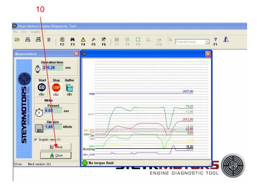
The setup button (10) calls the window for the graphic view setup.
