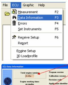
Menu "ECU -> Data Information" or the "F3" button on the toolbar calls the information window of the ECU. Here you can see the total engine runtime (1), the software version (2), the stored zero positions for the rack and the timing device (3) (timing device only for vehicle applications), if programmed the engine serial number (4) and the time the engine worked in the different modes (5).
