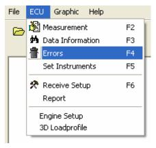
Menu "ECU -> Errors" or the "F4" button on the toolbar calls the window where every stored error code is shown. The probable reason of malfunction will appear in the red field (1) once you marked an error.
