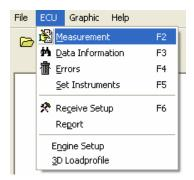
Menu "ECU -> Measurement" or the "F2" button on the toolbar calls the window for online measurements.
