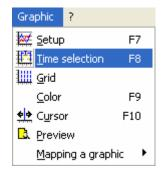
Using this window enables a feature which allows you to set the beginning and ending time of the logfile by moving the time cursors (1) with the scrollbars (2). This function is used to "zoom" into a specific area of the logfile by choosing the channel of interest (3).
