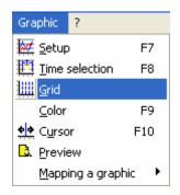
Using this functions enables and disables the grid in the graphic view and switches the background color from black to white.
