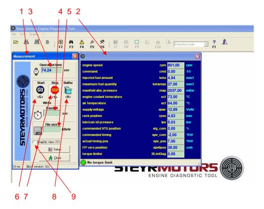
The button "Start" or hard key "G" (6) starts recording of engine data. The button "Stop" or hard key "S" (7) stops logging and calls the "save file as.." window, where a name for the recorded file (should be the engines serial for normal) can be typed in. With the button "Buffer" or hard key "B" (8), you activate a function that automatically stores the last 100 measuring points without the need to start logging first. It also calls the "save file as.." window immediately when pressed.
