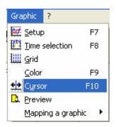
"Menu -> cursor" or the "F10" button on the tool calls the cursor control and measuring window. The value of every channel in the intersection of the cursor (1) is displayed in the line colored boxes (2).
