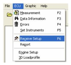
Menu "ECU -> Receive Setup" or the "F6" button on the toolbar calls the window for input parameter selection.
