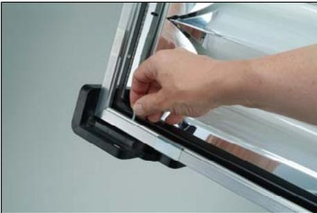
Align the pins of the Gel Frame with the **inner** (closest to lamps) holes of the Accessory Holder. Pull back the pins and release into the holes to secure the gel frame.
