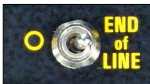
The **END of LINE** switch must be set to open ( **O** ) on Fixtures within the DMX chain.
