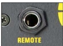
Lamps can be controlled manually through a hand held remote controller (**DIM-5**). For **Manual Remote Lamp Control** plug in the accessory **DIM-5**. Rotating the dimmer knob turns lamps on and off in sequence.
