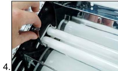
1) Open the two hinged reflector panels. 2 & 3) Insert the lamp base into the lamp connector. 4) Insert the lamp tip into the lamp clip. Close the reflector panels.
