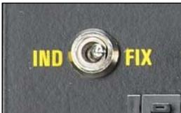
Setting the unit to "FIX" mode allows the user to re-create the "Inside-Out" pattern of the manual switch.
