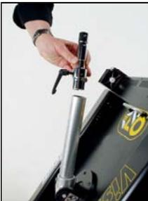
Remove the Junior Pin (**MTP-V63JR**) and attach the Hanging Adapter. It is held in place by a safety screw and a setscrew. A lock knob adjusts rotation of the arm.
