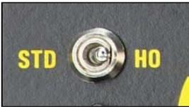
The VistaBeam 600's 7<sup>th</sup> DMX address controls the **STD/HO** function. The VistaBeam 300's 4<sup>th</sup> DMX address controls the **STD/HO** function.
