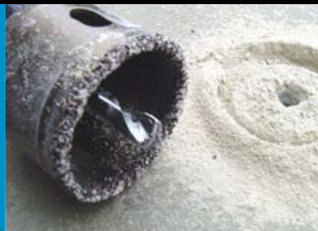
21779 Mandrel with carbide tip.
