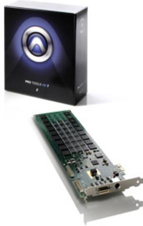
By combining the power of PCIe expansion through an EB4-1U-X8 system with multiple such PCIe cards, the same PC can record substantially more tracks. Additionally the same system may contain a storage controller (SAS/SATA/SCSI) and the hard drives for actually recording the tracks – all inside one box, freeing much of the PC hardware for other tasks.
