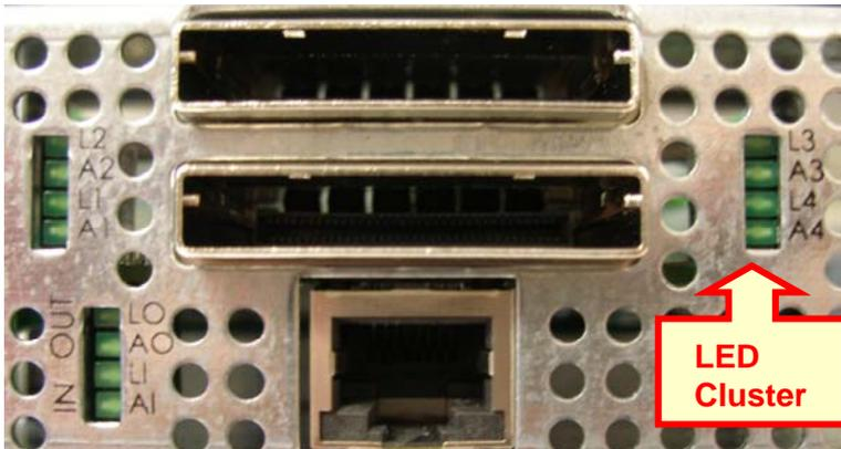
The three LED clusters display **Link (L)** and **Activity (A)** status for Uplink communication with the Host; Downlink communication with a Daisy- Chained chassis (see Appendix A for [Daisy-Chain setups](#)) and communication with the four PCIe expansion slots as follows:
