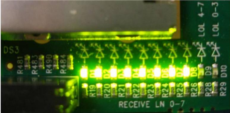
During normal operation all LEDs should be ON with the exception of D9 and D10, whose role is to indicate loss of signal. If the Host system is off, all LEDs should be off even if the chassis itself is turned on.
