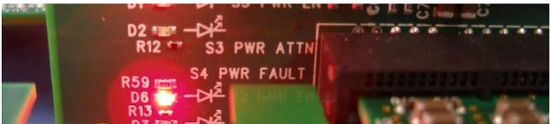
If the Host system is turned ON but there is no PCIe card in the slot, the Power Fault LED will be ON as well, as can be seen below:
