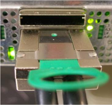
*Connect one end of the cable to the bottom iPass connector*
