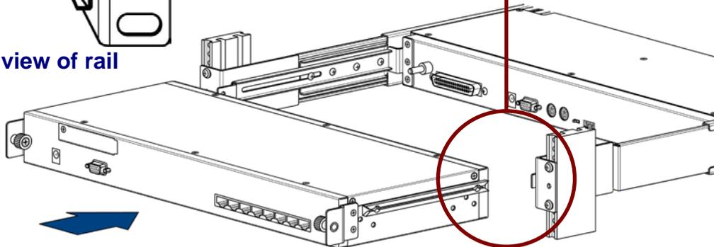
3. Tight thumb screw of bracket up to fix KVM switch in console (Both sides) and finish installation.
