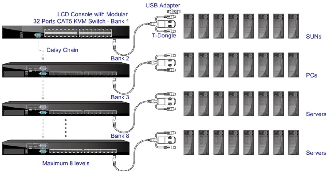
**Figure 2-9. Modular KVM Switch Daisy Chain Connection**
