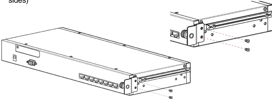
2. Push KVM switch into the rails from rear of console.
