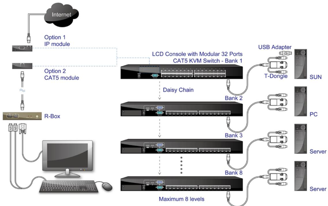
Figure 2-3. Computer / Server Installation
