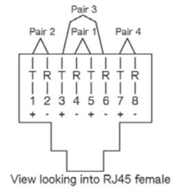
Figure 1-6. CAT5/5E/6 Straight Through UTP/STP Cable (8P8C)
