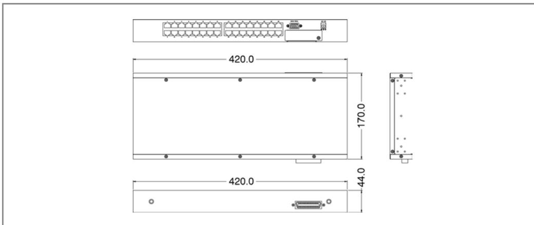
**Figure 1-2. Mars 8D / 16D / 32D Series Dimensions**
