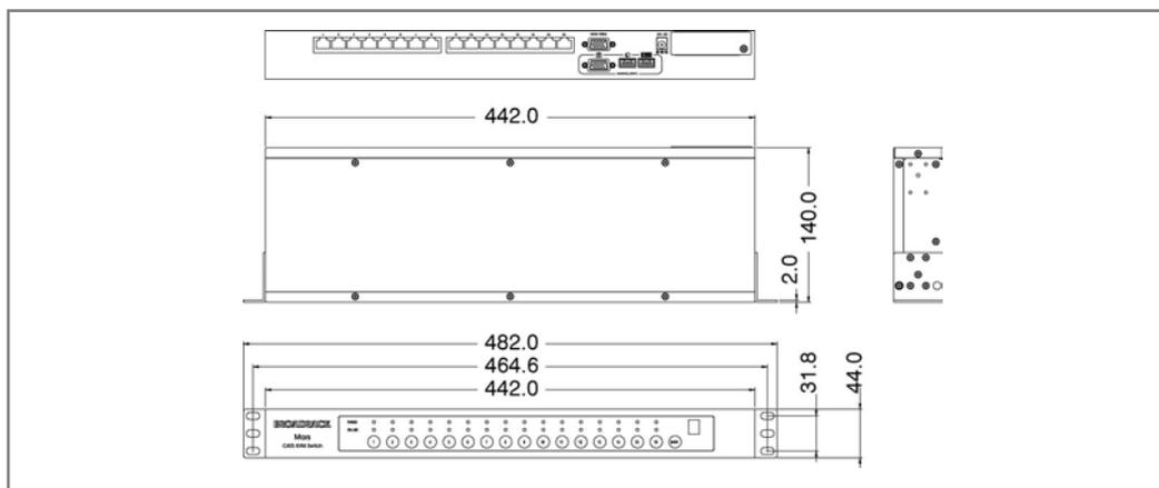
**Figure 1-1. Mars 8 / 16 Series Dimensions**
