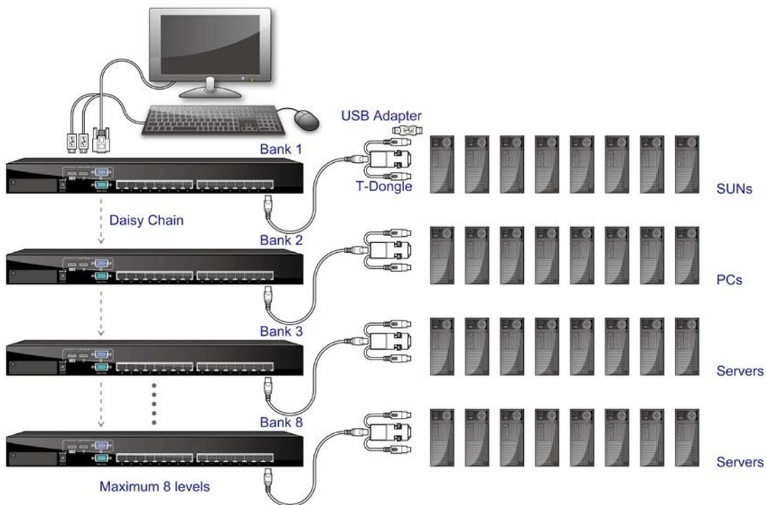
Figure 2-8. Stand Alone KVM Switch Daisy Chain Connection
