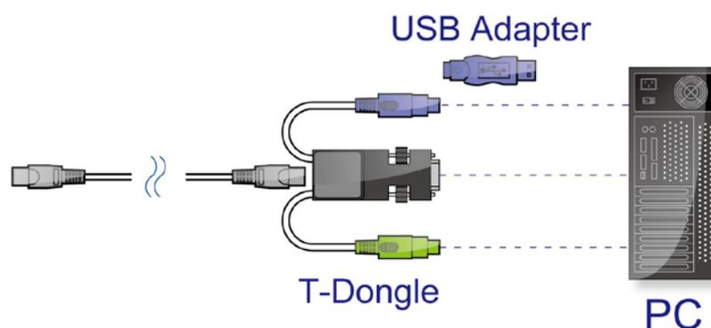
Figure 2-4. PS/2 T-dongle and PS/2 to USB adapter
