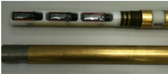
3 x 9 v Lithium batteries
