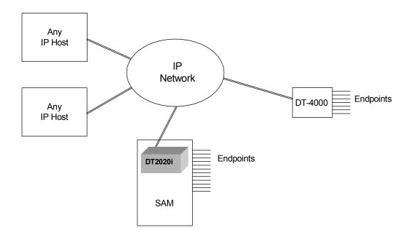
The above configuration is not the only possible one. However, it does depict some of the networking capabilities of this device. A port on a SAM with a DT-2020i could be having a session directly with an IP host. A second port on the same SAM could be having a session directly with a device connected to a DT-4000. A third port could be connected to a fourth port on the same SAM, since local switching is done at the DT-2020i.
