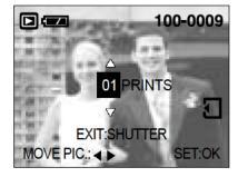
4. Once the DPOF setting is finished, the number of prints will be displayed at the left side of the LCD monitor. The number of prints that can be set is between 0 and 30. If you select '0(zero)', you can't print an image.
