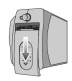
2. Have the front of the memory card facing toward the front of the camera (lens) and the card pins toward the back of the camera (LCD monitor), and then push the memory card into the card slot until you hear a click.
