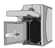
To close, push the card cover until you hear a click. If the memory card does not slide in smoothly, do not attempt to insert it by force. Check the direction of insertion, and then insert it correctly.
