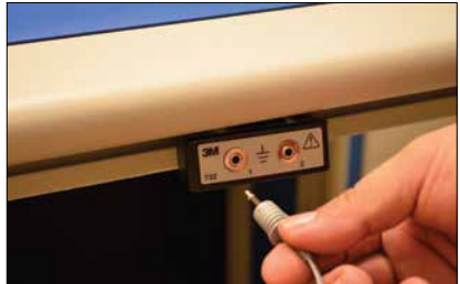
Figure 13 – Connecting wrist snap ground cord to 3M™ Dual Conductor Remote Input Jack Model 732.
