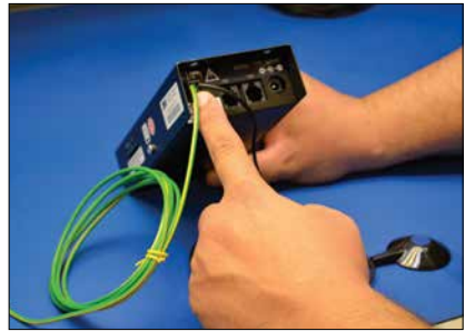
Figure 8 – Inserting two-wire connector into rear of 3M™ Workstation Monitor Model 724.
