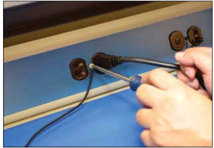
Figure 7A – Attaching system grounds. Note work, surface and unit are grounded at different locations.
