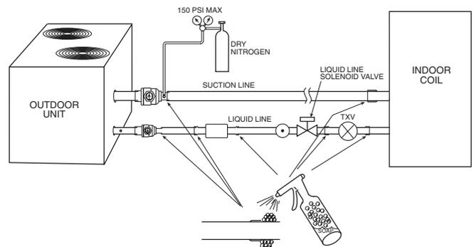
**→ Fig. 16 — Recommended Process for Checking for Leaks**
