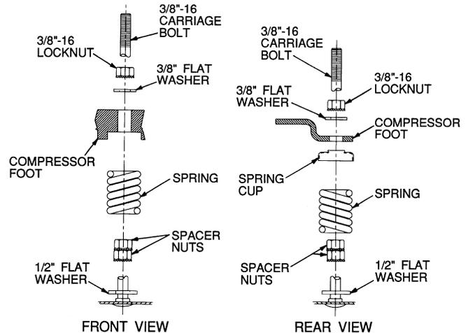
**Fig. 15B — Compressor Mounting — 541A180 Units**
