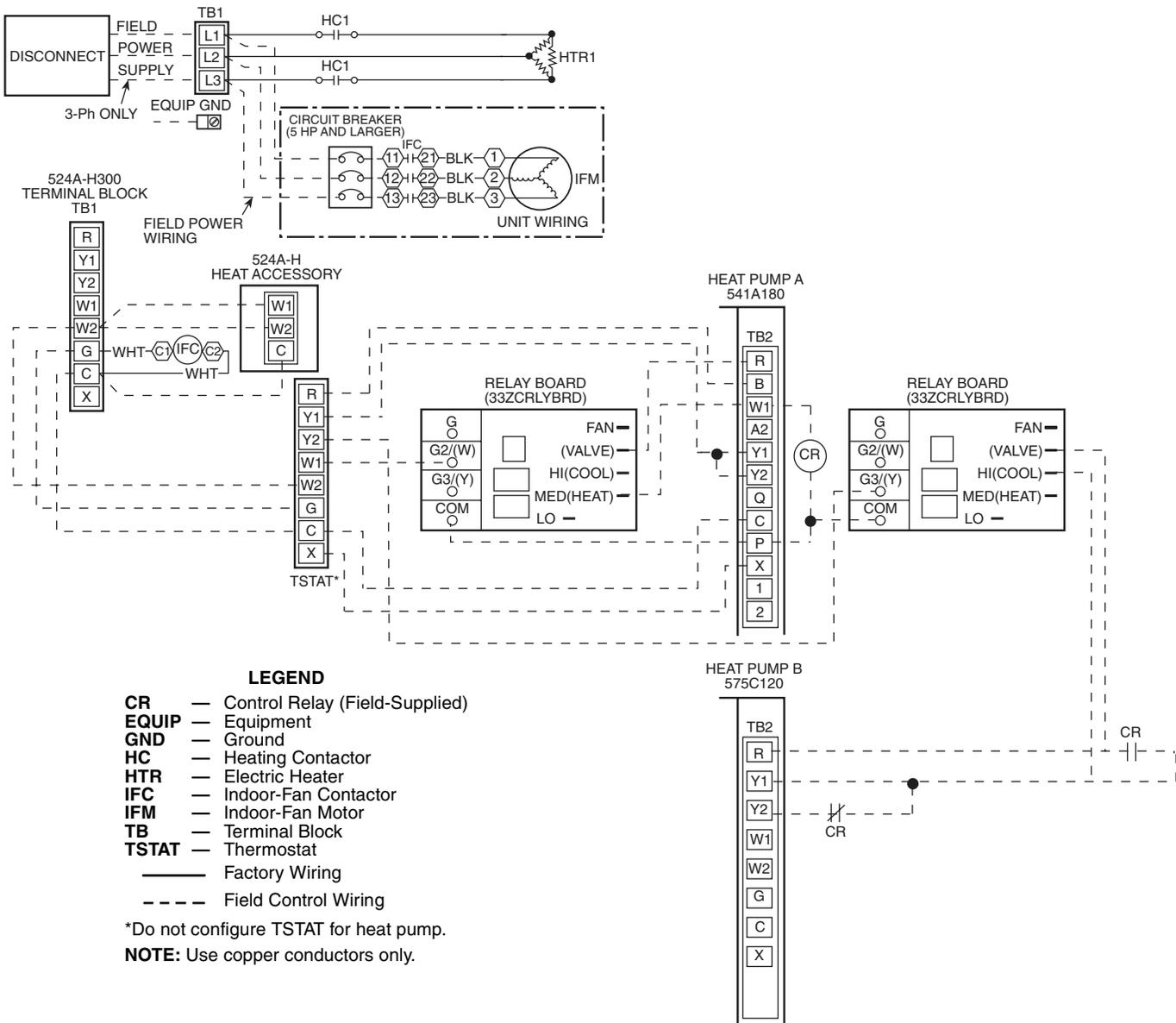
Fig. 13 — Wiring Diagram — Duplex 575C120 and 541A180 With 524A-H300 and Electric Heat
