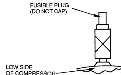
**Fig. 6 — Location of Fusible Plug — 541A180 Unit**
