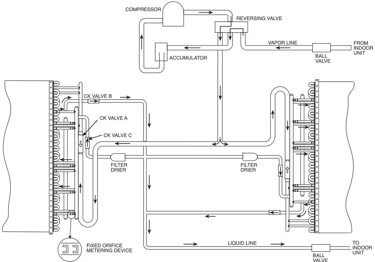
Fig. 20 — 575C090,120 Cooling Mode (Size 090 Shown)
