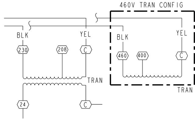
**Fig. 8 — Wiring Diagram — 575C090,120 — Control Transformer**
