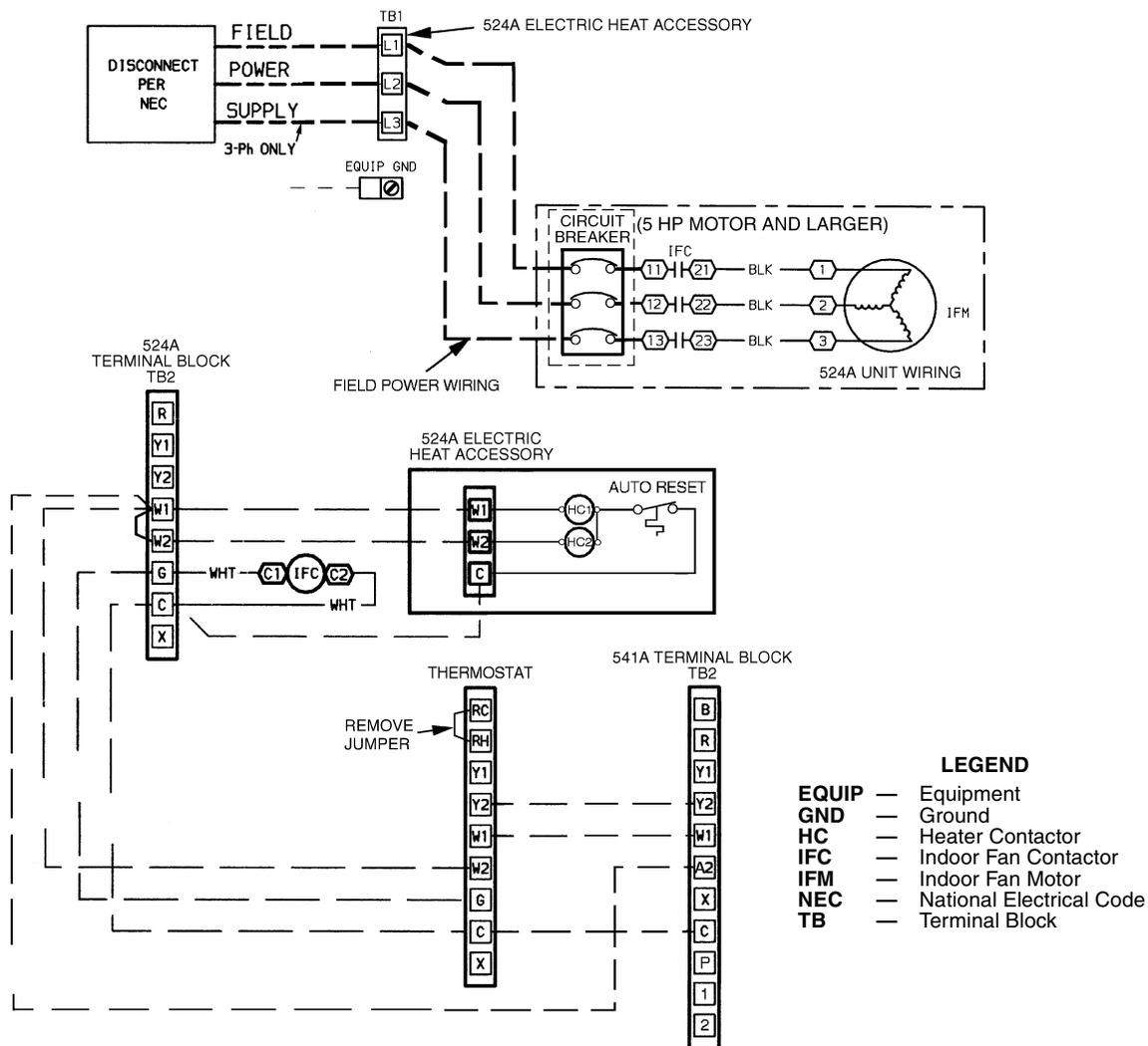
Fig. 11 — Wiring Diagram — 541A180 Unit With Standard Thermostat and Electric Heat
