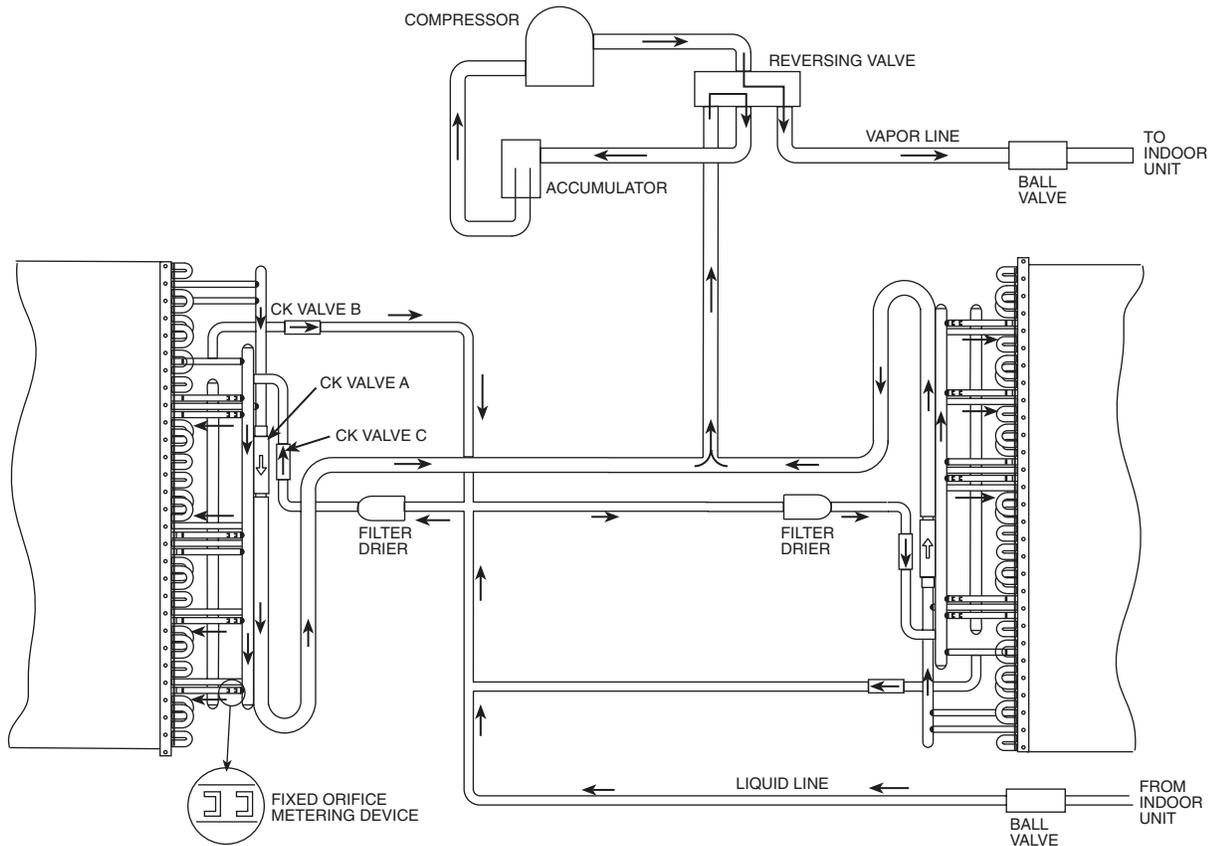
**Fig. 21 — 575C090,120 Heating Mode (Size 090 Shown)**
