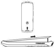
2 Insert battery as shown below. Push the battery down until it snaps in place.
