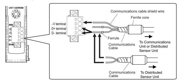
To prevent the communication cable from becoming disconnected, install a rod terminal.
