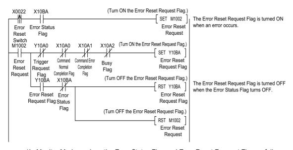
\*In Monitor Mode, replace the Error Status Flag and Error Reset Request Flag as follows: Error Status Flag: Change X10BA to X11BA. Error Reset Request Flag: Change Y10BA to Y11BA.
