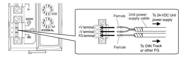
Securely attach ferrules to the Unit power supply cable wires. Do not wire a power supply to the communications path of the Distributed Sensor Units. The Units may be damaged.
