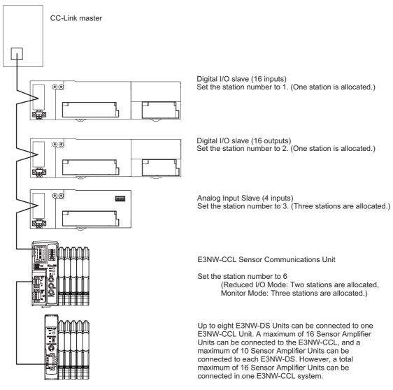
The Unit power supply and I/O power supply are not shown in the above figure. They must be provided separately.
