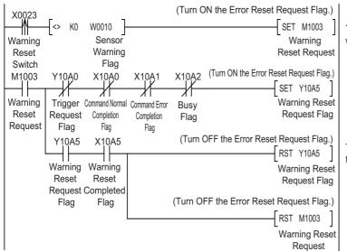
The Warning Reset Request Flag is turned ON when a warning occurs (i.e., when the Warning Flag is not 0).
