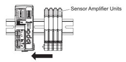
4 Secure the enclosed DIN Track End Plates (PFP-M) onto the ends so that there is no space between them and the Units. Finally, attach the protective cap you removed in step 3 to the Sensor Amplifier Unit on the far right end.
