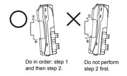
After you have completed the above procedure, check to make sure that the E3NW-CCL is mounted securely into place.
