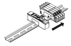
**2** Press in on the Distributed Sensor Unit toward the DIN Track and lift up to remove it.
