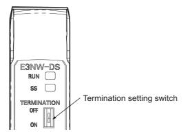
Turn ON the DS-Bus termination setting switch for the last Distributed Sensor Unit on the DS-Bus network. Turn this switch OFF for all other Distributed Sensor Units. This is shown in the following figure.
