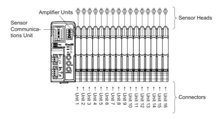
Example 2: Connecting a Communications Unit and Distributed Sensor Units
