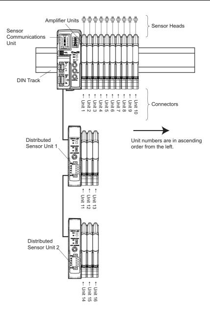
The Sensor Communications Unit identifies the connected Sensor Amplifier Units according to their unit numbers.
