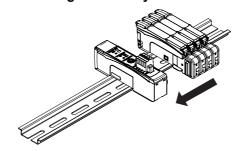
4 Secure the enclosed DIN Track End Plates (PFP-M) onto the ends so that there is no space between them and the Units. Finally, attach the protective cap you removed in step 3 to the Sensor Amplifier Unit on the far right end.
