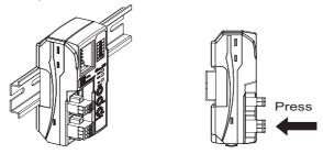
Remove the protective cap from the right side of the Sensor Communications Unit. Then, slide the Sensor Amplifier Unit, align the connector with the Sensor Communications Unit, and press the Units together until you hear them lock into place.
