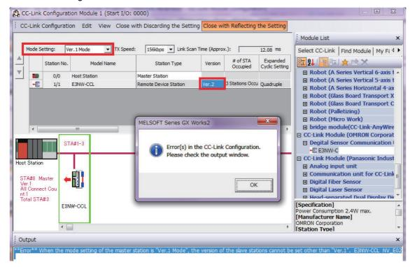
If the above error message is not displayed but communications are still not working (i.e., the RUN indicator on the E3NW-CCL does not light up), check to confirm that the switches for the baud rate, operating mode, and station number are all set correctly based on the parameters set for the master station.
