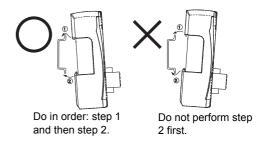
After you have completed the above procedure, check to make sure that the E3NW-DS is mounted securely into place.
