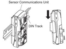
Press the bottom part of the Unit onto the DIN Track.
