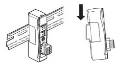
**2** Press the bottom part of the Unit onto the DIN Track.
