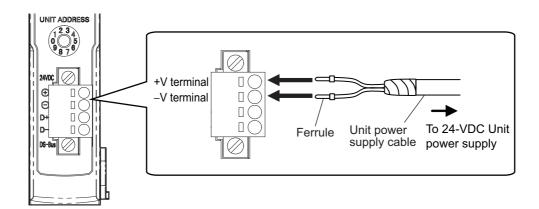
Securely attach ferrules to the Unit power supply cable wires.
