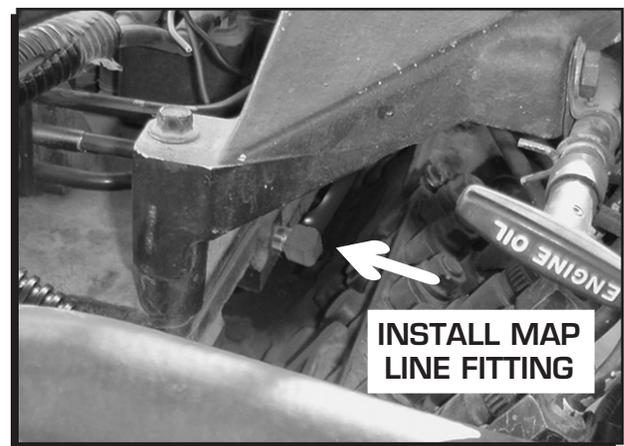
Figure 5 Connecting the MAP Sensor.
