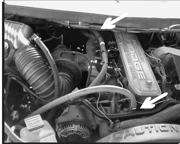
Figure 6 Installing the Coolant Hoses.
