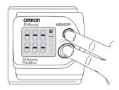
2 Press Memory Recall button and simultaneously On/Off button to erase memory.
