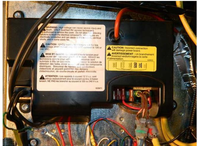
**Fig. 12 Typical Norcold Power Terminals**
