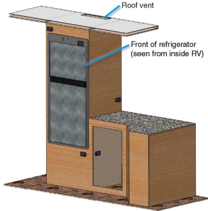
**Fig. 3 Typical Inside View of Refrigerator Installation**
