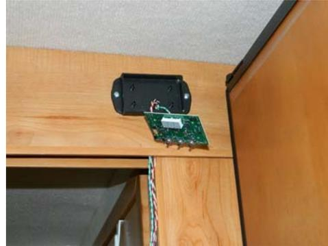
**Fig. 7 Mount Housing & Route Wires**
