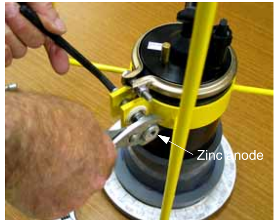
Figure 7-3: Loosening the Zinc Anode
