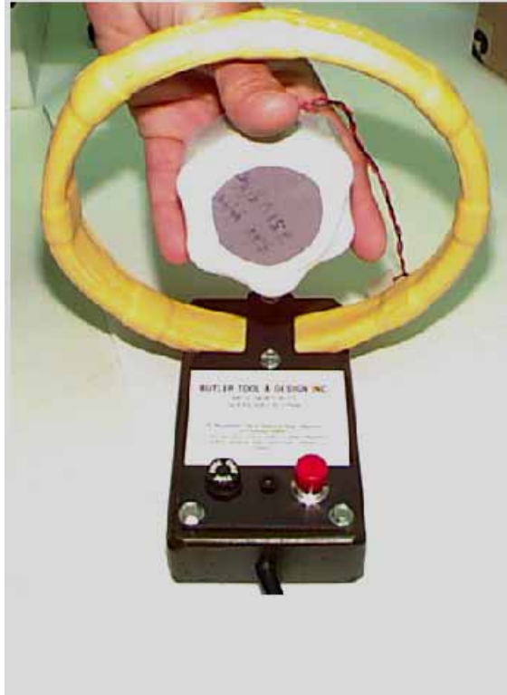
Figure 7-1: Degaussing a Battery Pack with a Degaussing Coil
