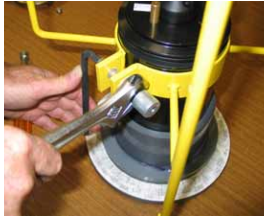
Figure 7-5: Loosening the Nut and Bolt Securing the Mooring Frame
