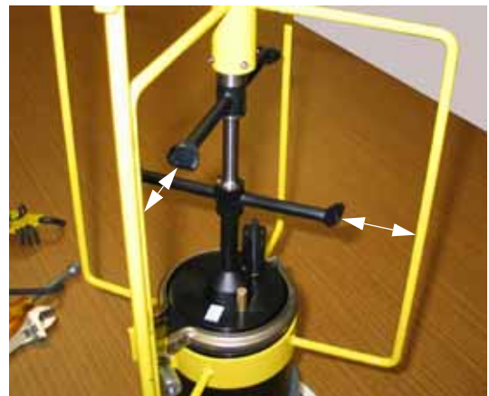
Figure 7-9: Aligning Fingers of Velocity Head with Mooring Frame
