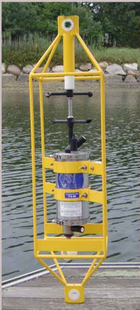
7000-meter 2D-ACM with the optional 5-ton mooring frame
